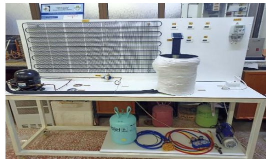
Figure 2. Vapor compression refrigeration system test rig
