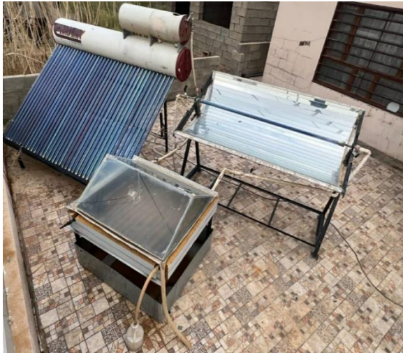
Fig. 1. Experiment set up of active solar still coupled with ETC and PTC.
