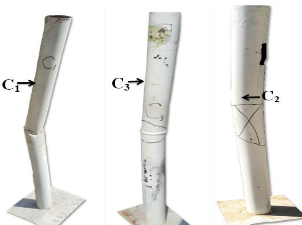
Figure 7. Patterns of failure for circular W.C.F.S.T columns subjected to axial loading.
