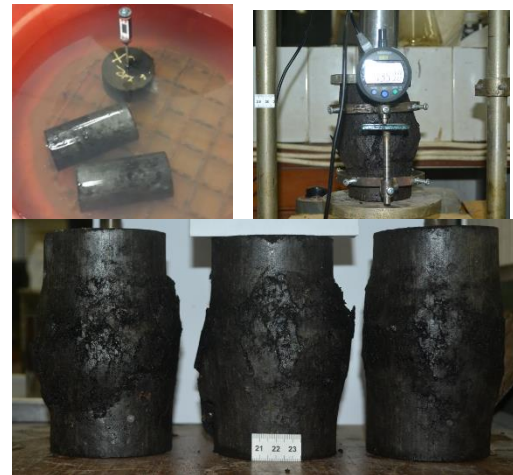
Figure 6. (a) Specimen immersion; (b) specimen UCS test; (c) specimen after UCS test
