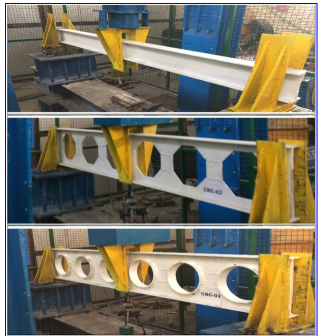
Figure 5: Test Setup for Specimens
