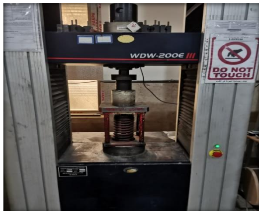
Figure 5. Experimental setting of deep drawing process
