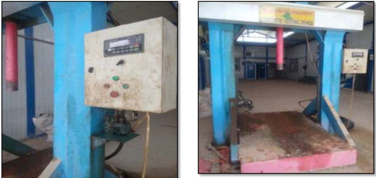
Figure 2: Universal test machine used in experimental tests.
