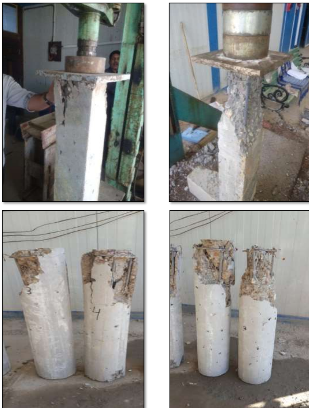
Figure 3: Failure modes of square and circular short columns
