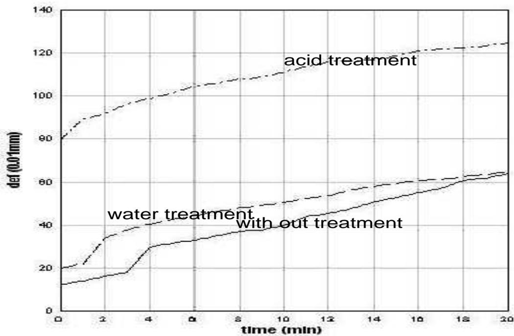
Figure 14 the variation of Central deflection with time for tiny corn composites
