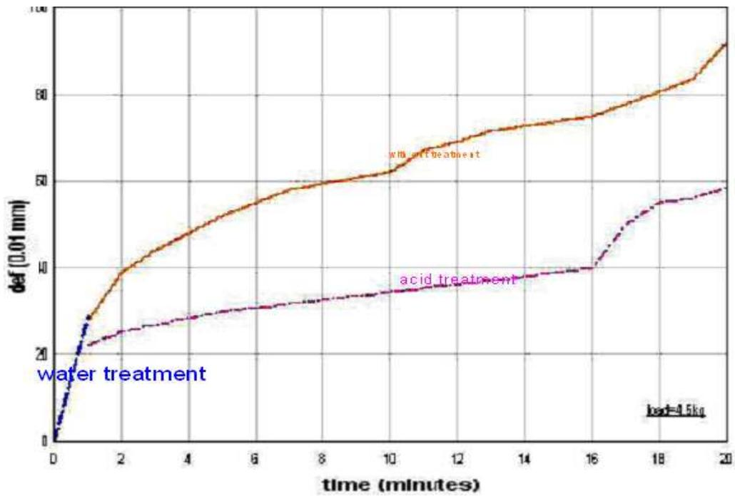
Figure 11 the variation of Central deflection with time for starch composites
