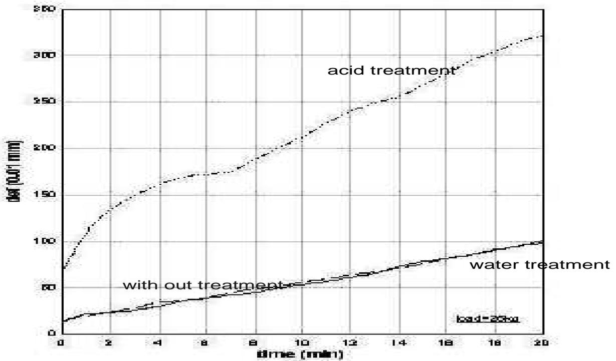
Figure 9 the variation central deflection with time for fiber glass composites the variation
