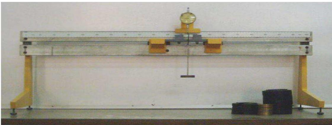
**FigureB.1** bending test apparatus
