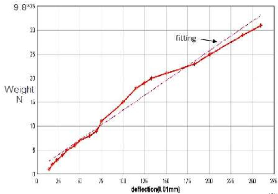
**Figure 1** the variations of the central displacements with load for fiber glass composite beam
