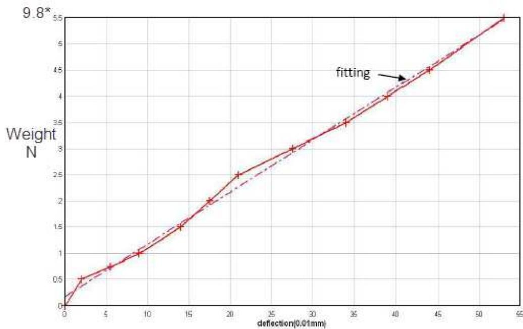
**Figure 3** the variations of the central displacements with load for starch composite beam.
