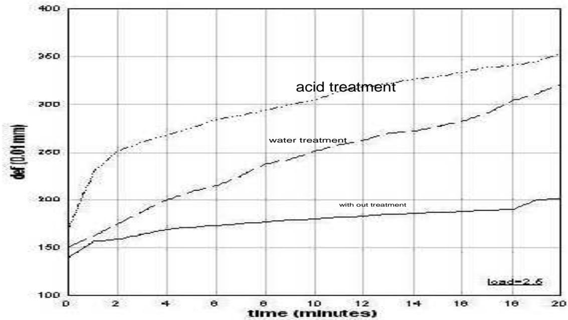
Figure 10 the variation of Central deflection with time for jute composites
