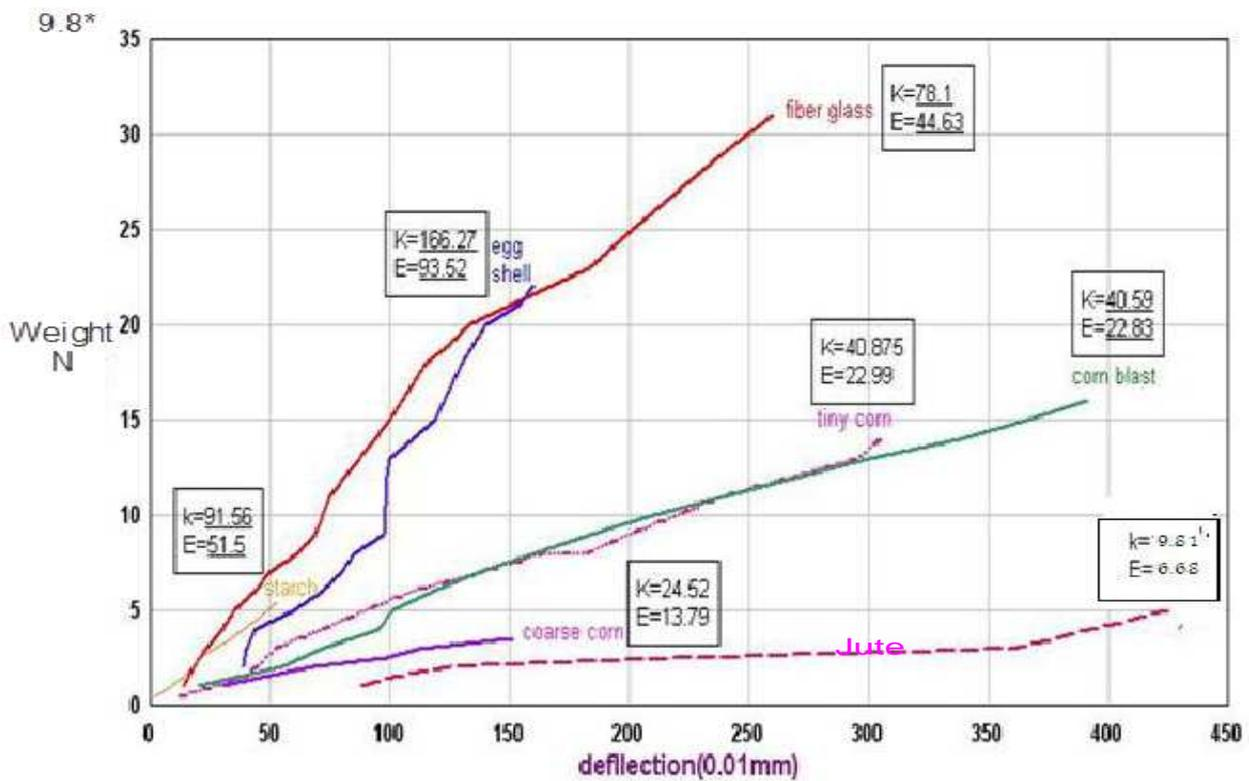
Figure 8 the comparison of bending behavior for many types of composites materials and their modulus of Elasticity (E) (MPa) and stiffness value (K) (N/mm).
