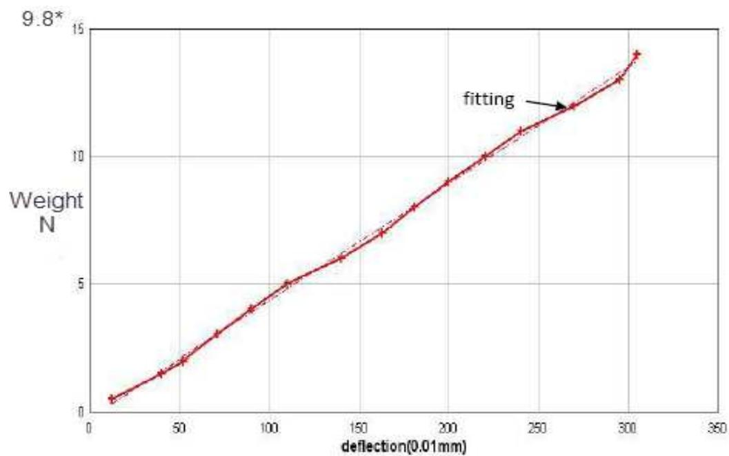
**Figure 4** the variations of the central displacements with load for tiny corn composite beam.
