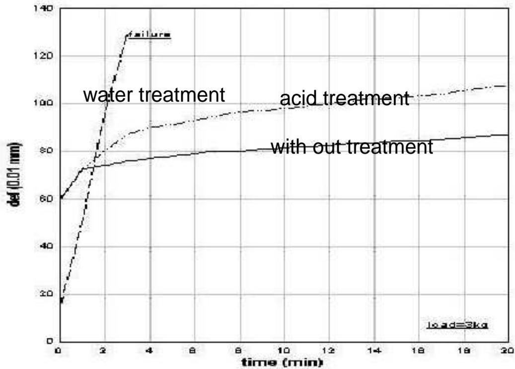
Figure 13 the variation of Central deflection with time for coarse corn composites
