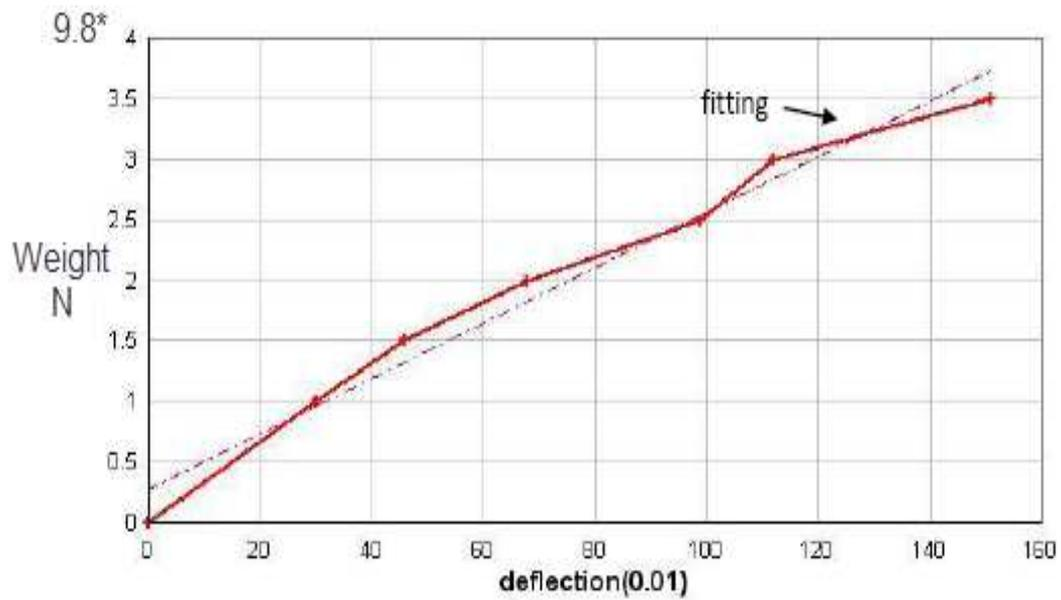
**Figure 5** the variations of the central displacements with load for coarse corn composite beam.
