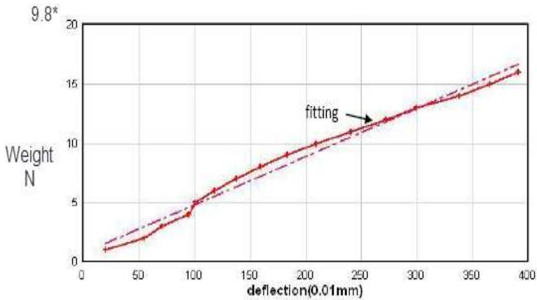
Figure 7 the variations of the central displacements with load for corn bast composite beam.
