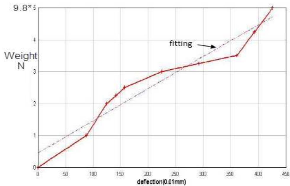
**Figure 2** the variations of the central displacements with load for jute composite beam.
