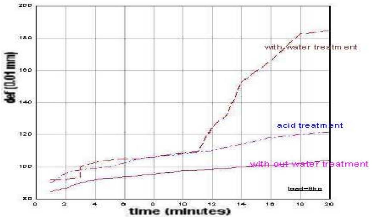
Figure 12 the variation of Central deflection with time for egg shell composites
