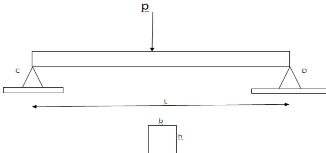
**Figure A.2** Show the simply supported beam with concentrated load
