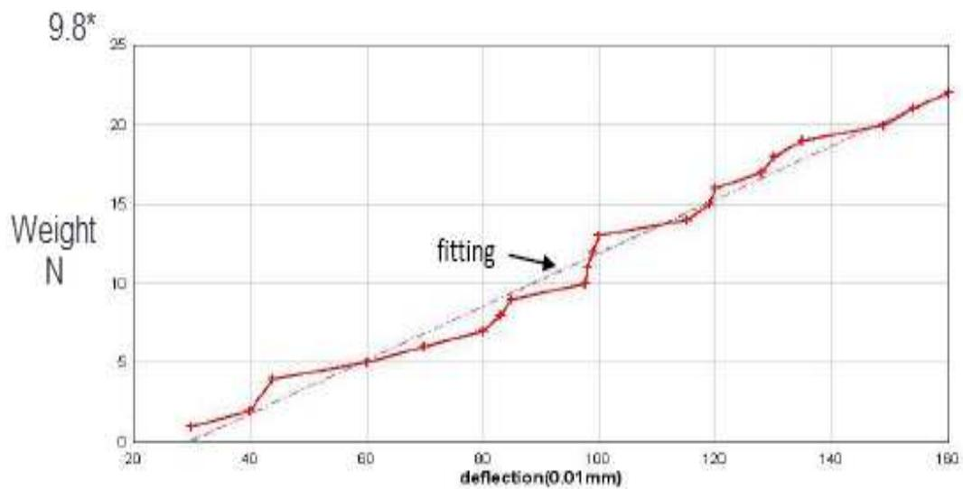
**Figure 6** the variations of the central displacements with load for egg shell powder composite beam.
