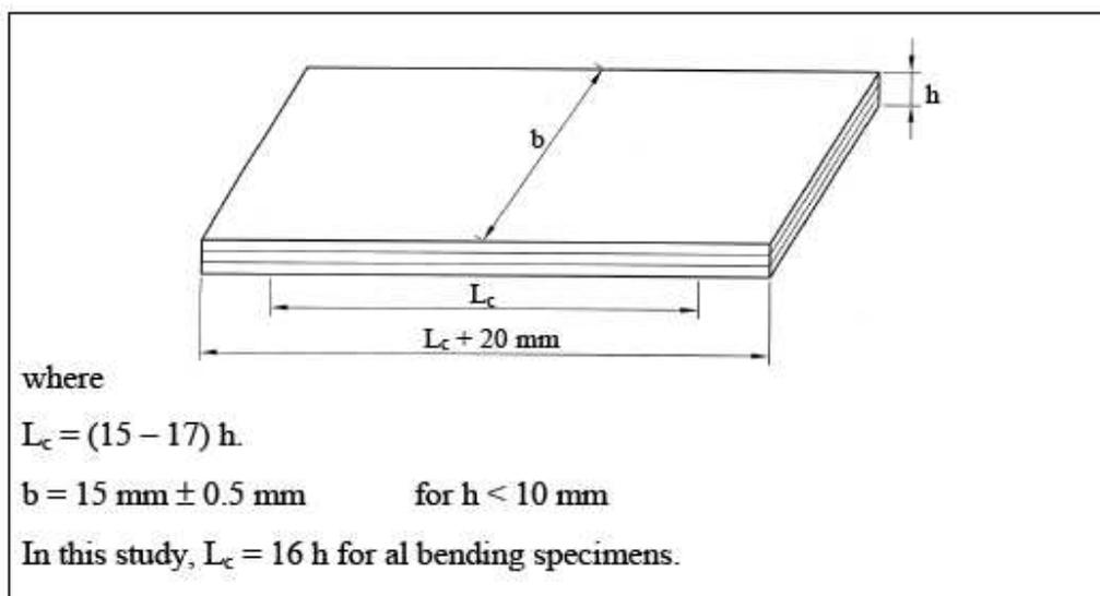
**Figure B.2** Bending specimen's dimension [8]
