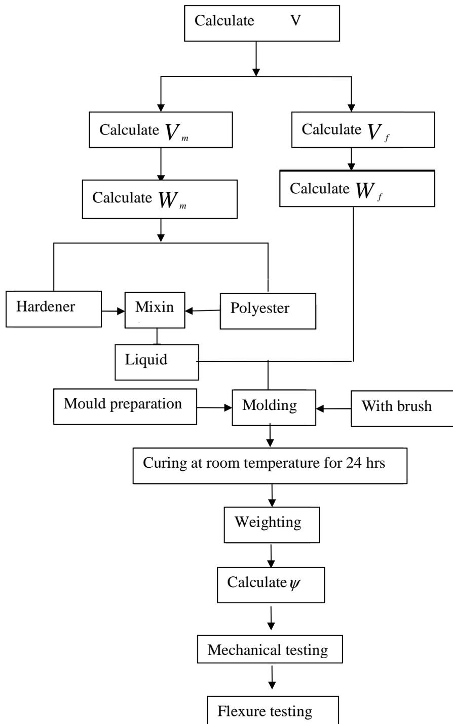
Figure B.3 show the flow chart of the steps of the sample preparation
