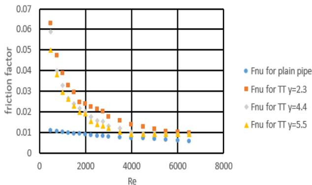
Figure 8. Numerical solution of friction factor for three twist ratios and plain pipe.
