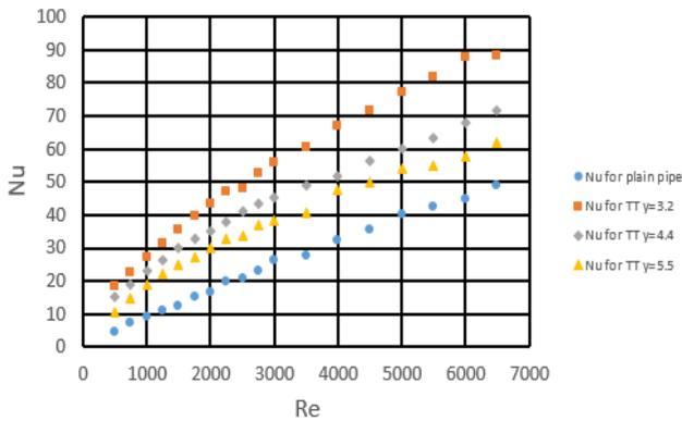
Figure 7. Numerical solution of Nusslet number for three twist ratios and plain pipe.
