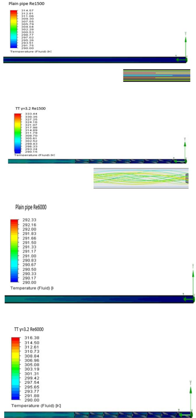
Figure 9. Comparison of the temperature distribution between plain pipe with that corresponding with a twist tape for  $\gamma=3.2$ .
