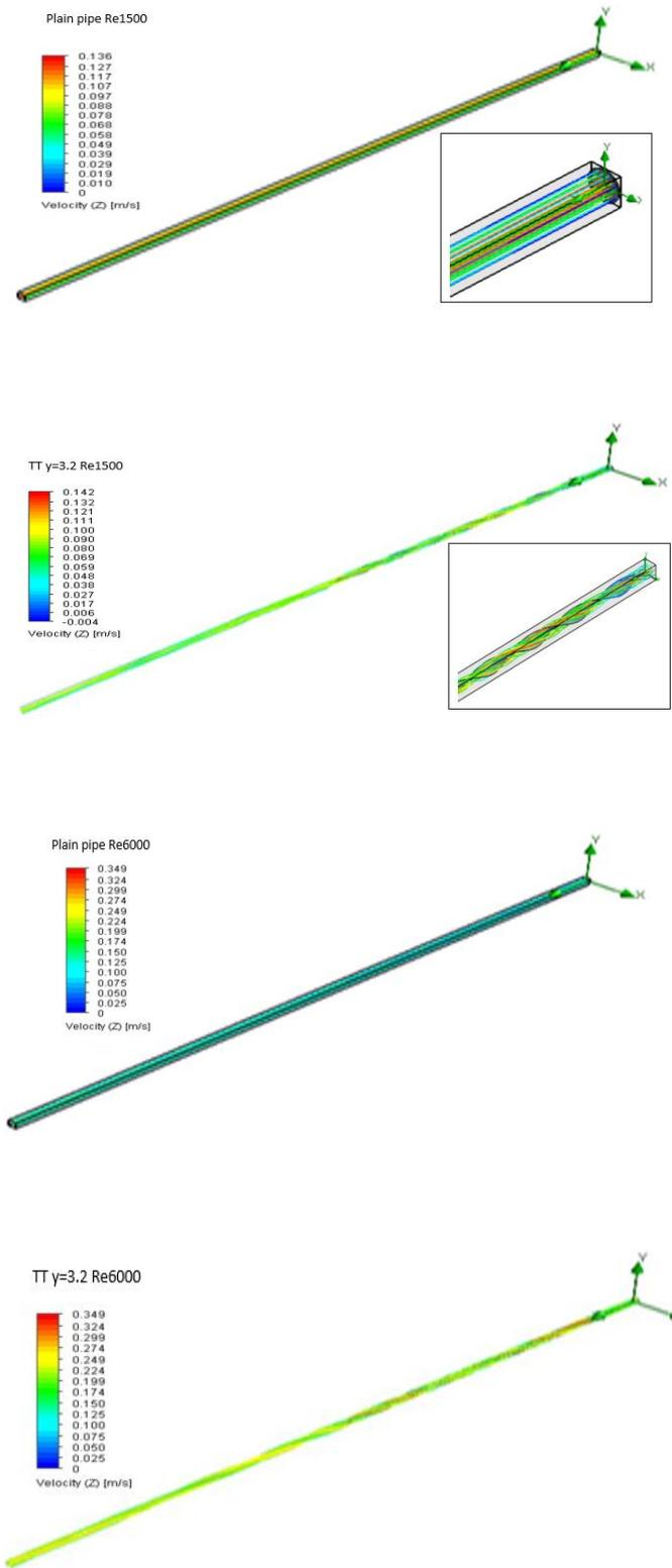
Figure 10. Comparison of trajectory of flow (identified by z-velocity) between plain pipe with that corresponding with a twist tape for  $y=3.2$ .
