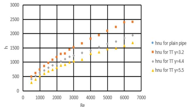
**Figure 4. Numerical solution of heat transfer coefficient vs. Reynolds Number for plain pipe, y=3.2, y=4.4 & y=5.5.**
