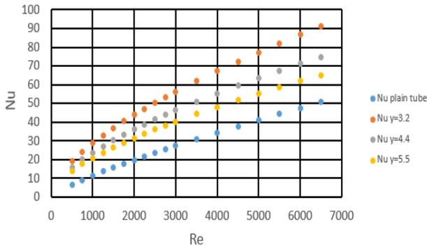
Figure 6. Theoretical solution of Nusslet number for plain tube and the three twist ratios.
