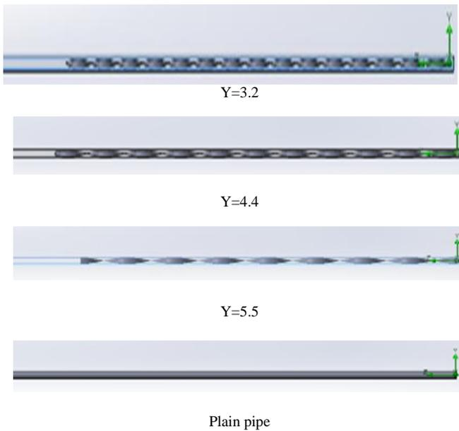
**Figure 3. Plain pipe and pipe include twist tapes with three twist ratios.**
