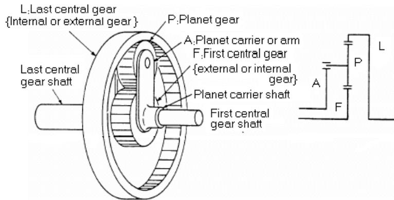
Figure 2 PGT of the lower arrangement.
