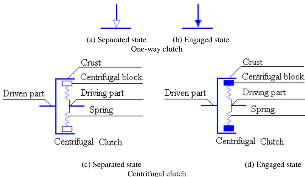
Figure 8 One-way clutch and centrifugal clutch in the engaged and separated states.
