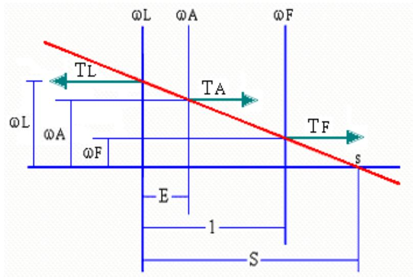
**Figure 5** Nomograph with torques represented as vectors perpendicular to the rotational speeds axes.
