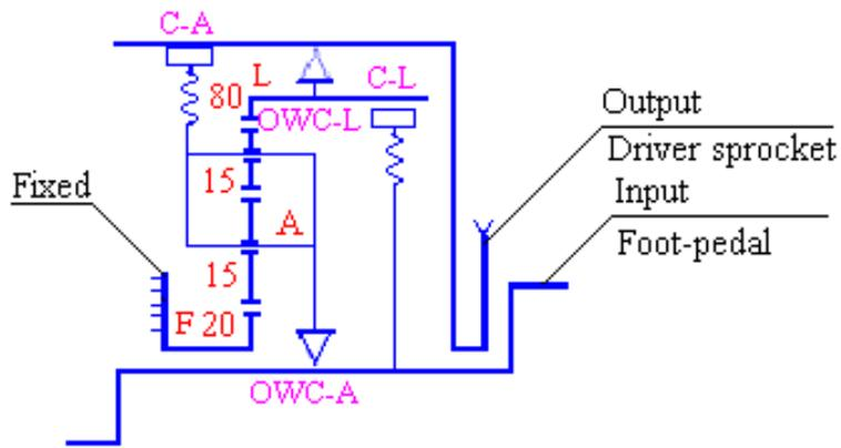
Figure 18 Design 3 for the bicycle three-speed automatic changer.
