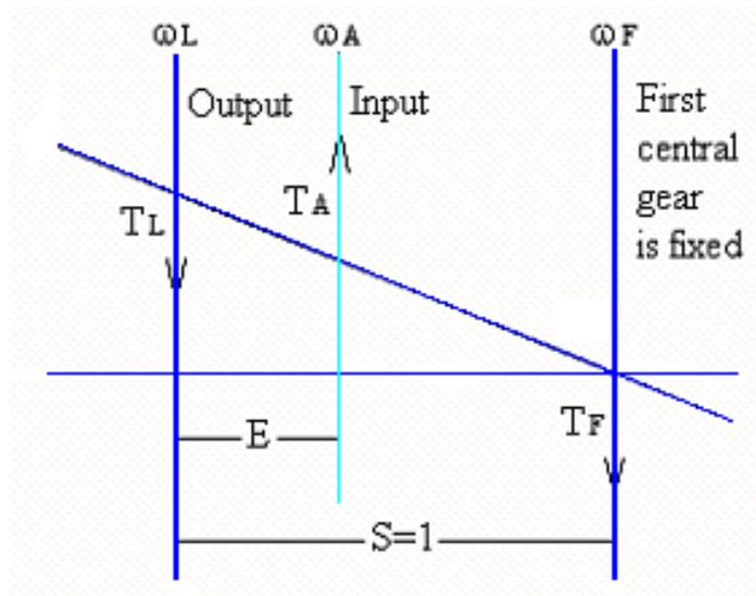
Figure 7 Nomograph for the PGT.
