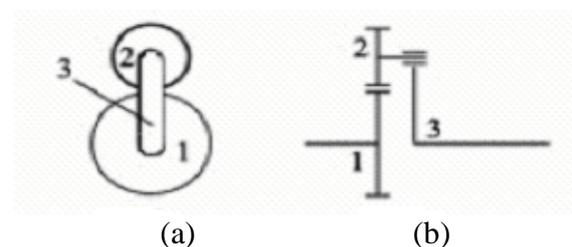
**Figure 1** (a) The elementary PGT and (b) its kinematical representation.
