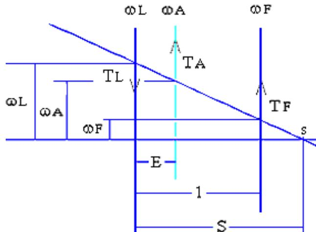
Figure 6 Nomograph with torques represented as vectors along the three axes.
