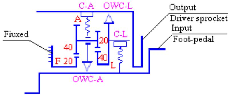
Figure 16 Design 2 for the bicycle three-speed automatic changer.
