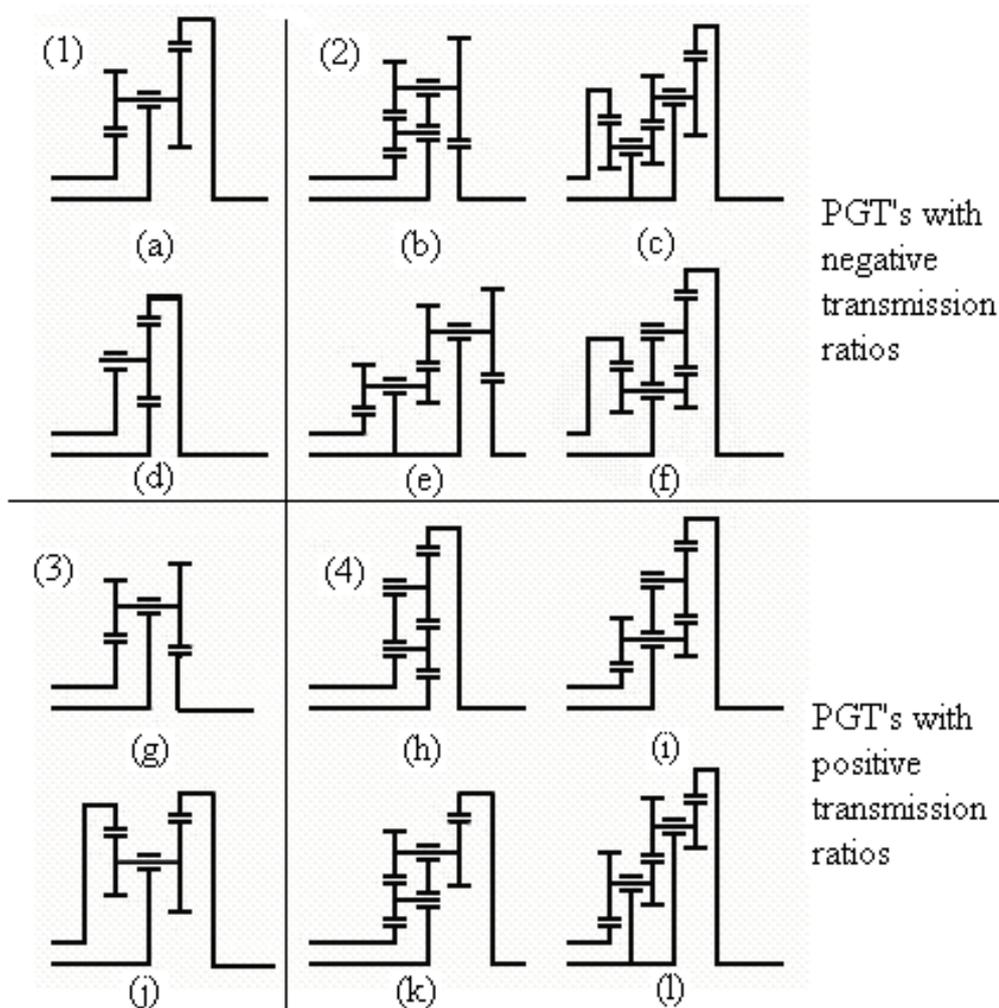
Figure 3 The simple, compound and complex PGT's as originally presented by Lévai.
