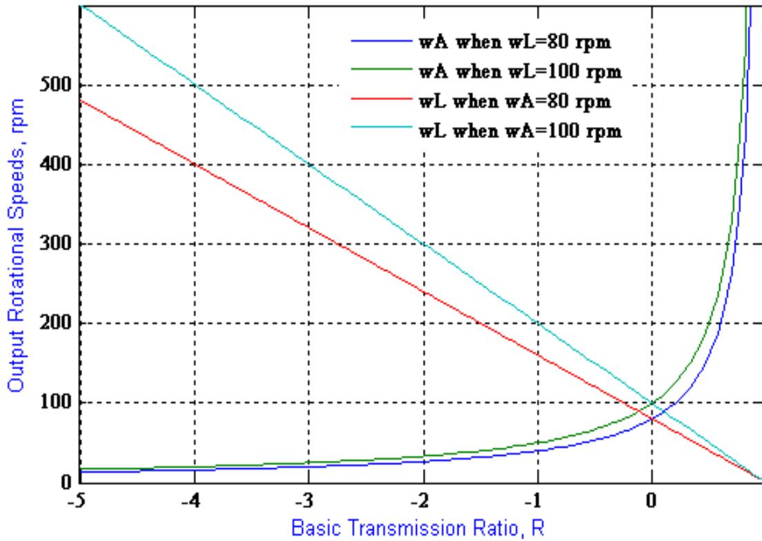
Figure 12 Output rotational speeds  $\omega_A$  and  $\omega_L$  as a function of train ratio R, for two pedaling speeds 80 and 100 rpm
