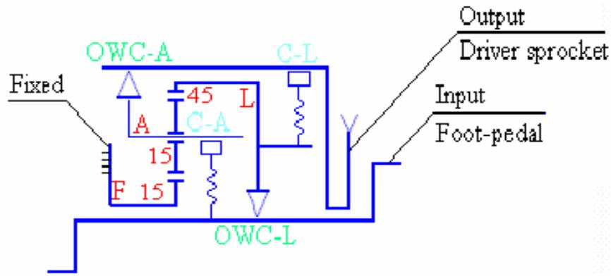
Figure 14 Design 1 for the bicycle three-speed automatic changer.
