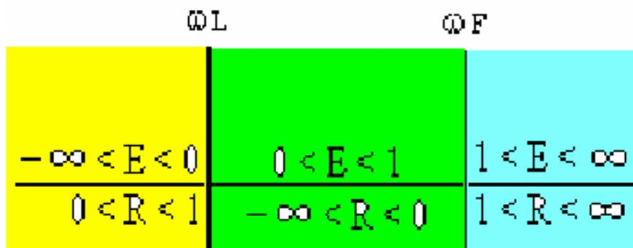
Figure 10 Nomograph with ranges of basic transmission ratio R labeled.
