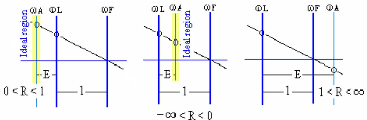
Figure 11 Nomographs for the system for the three ranges of R with ideal regions.
