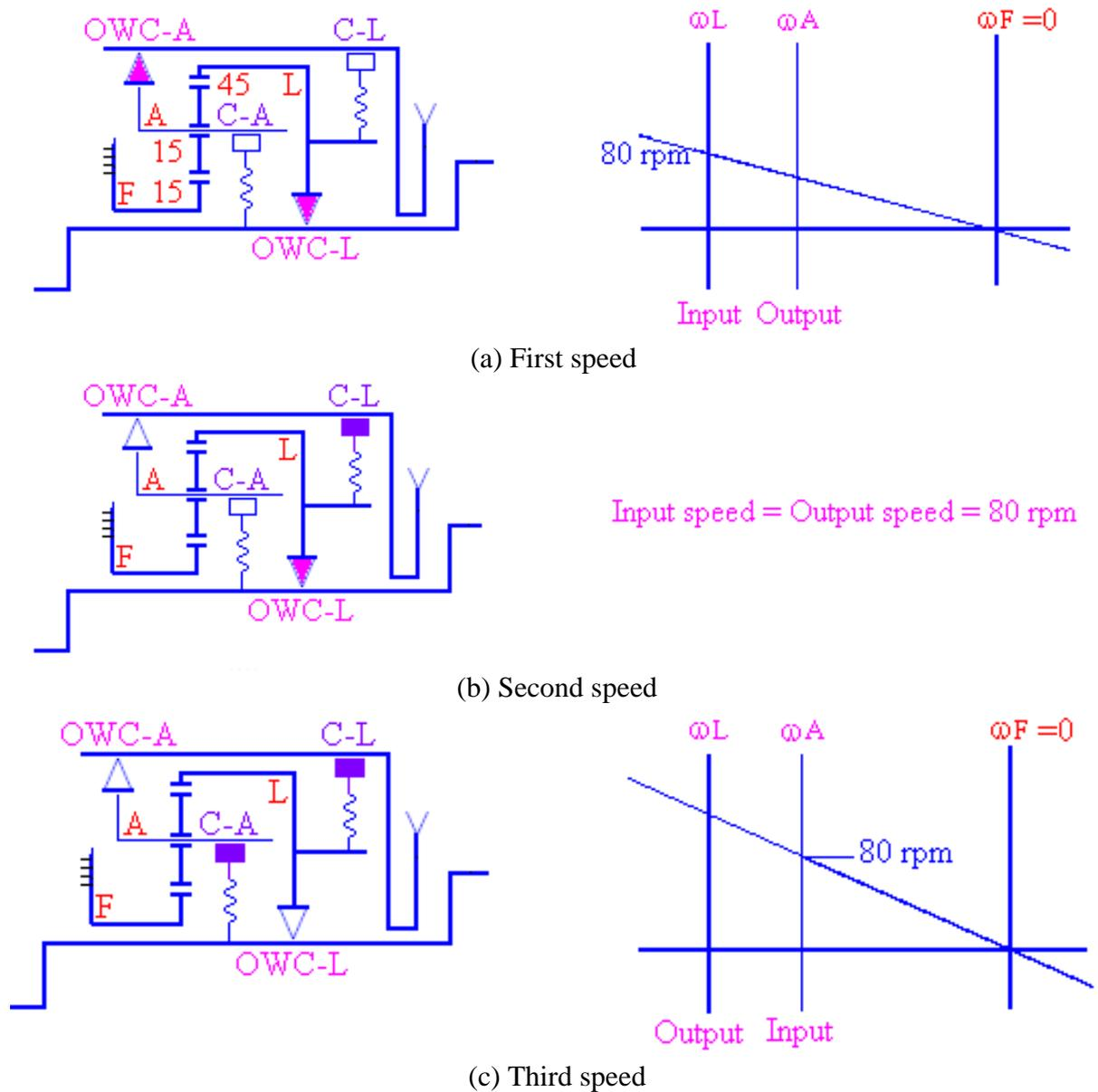
Figure 15 The three speeds of the speed changer of plan 1.
