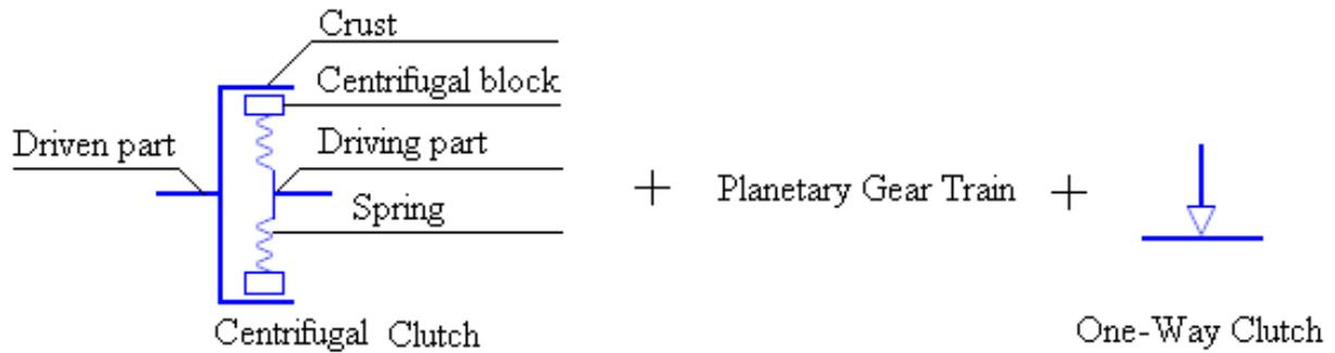
Figure 9 The automatic internal speed changer design.
