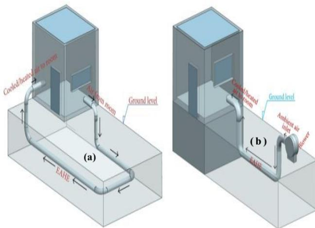
Figure 1. EAHE: (a) open loop and (b) closed loop [23]
