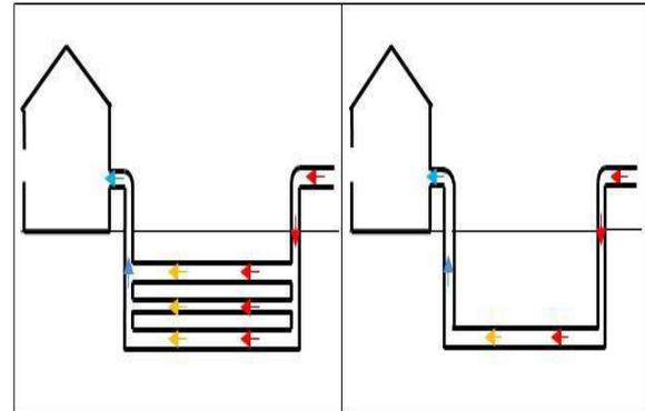
Figure 3. (a) Single tubes and (b) multiple tubes ETHE [25]
