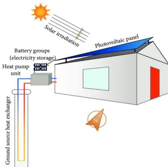
Figure 2. Solar-assisted ground source heat pump [24]
