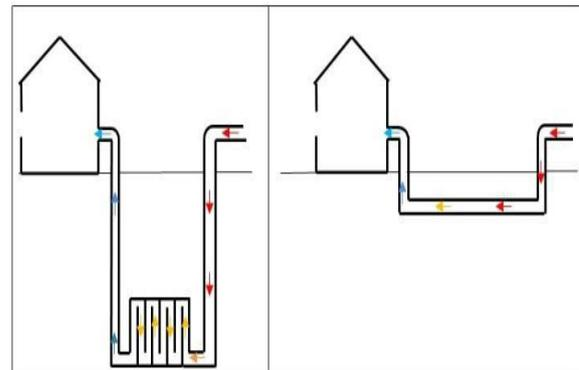
Figure 4. (a) Vertical and (b) horizontal ETHE [23]
