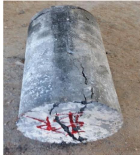
**Figure 2 - Splitting failure of RPC**
