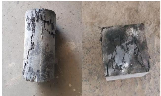
**Figure 1 - Compression failure of RPC cylinders and cubes.**
