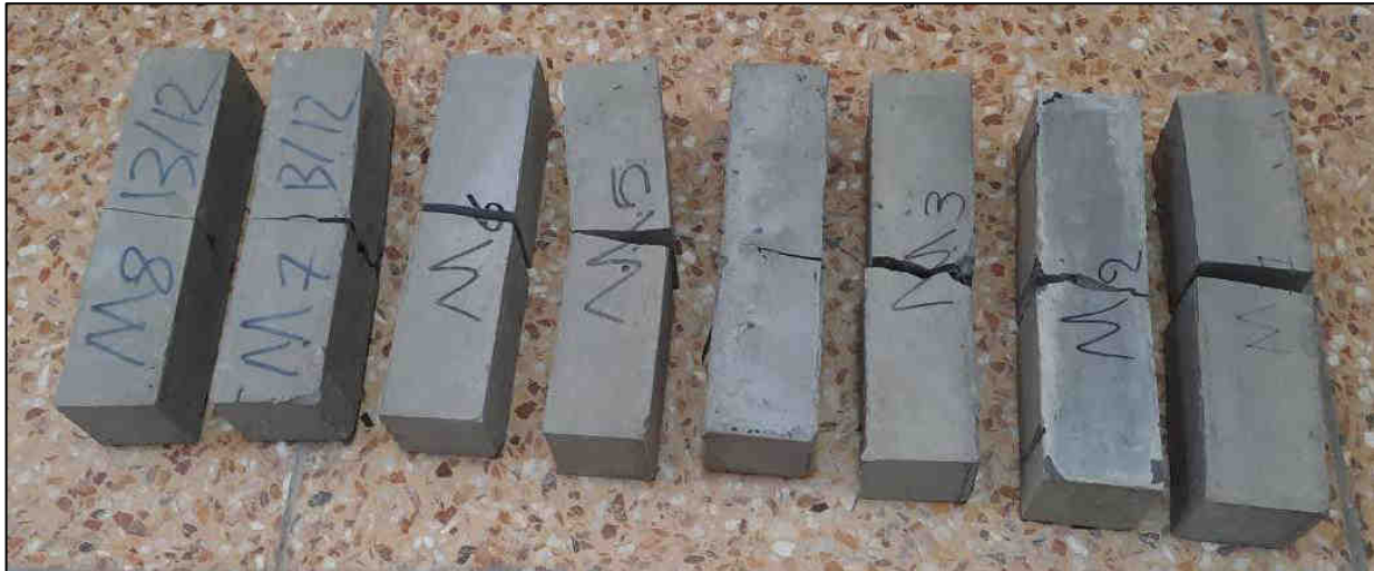
Figure 14. The broken prism specimens after the test
