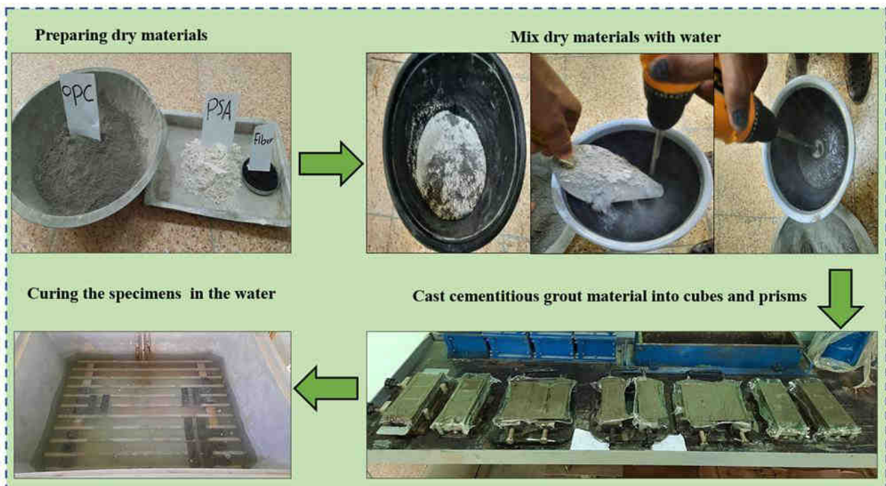
Figure 8. The cementitious grout preparation
