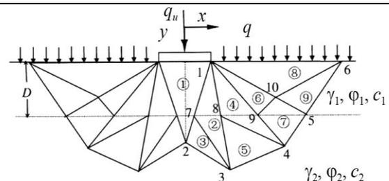
Figure 1: The suggested Huang and Qin (2009) failure mechanism.
