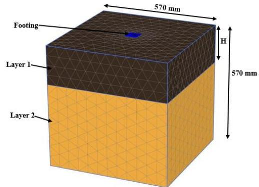
Figure 5: The model geometry and meshing for two-layered soil.
