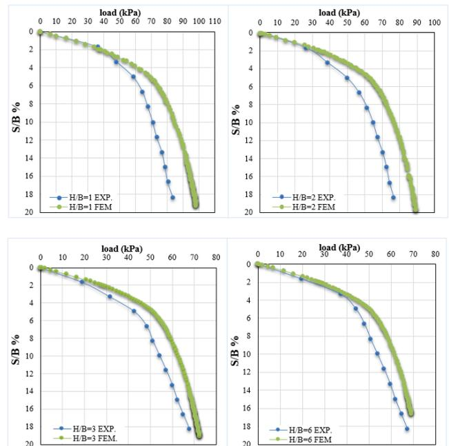
Figure 7. The experimental and numerical load-settlement curve of sand over clay layered.
