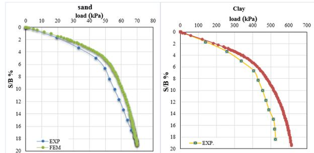
Figure 6. The experimental and numerical load-settlement curve of one layer of soil.
