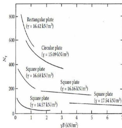
Figure 9. Variation of  $N_\gamma$  with  $\gamma B$  (adapted after DeBeer, 1965)
