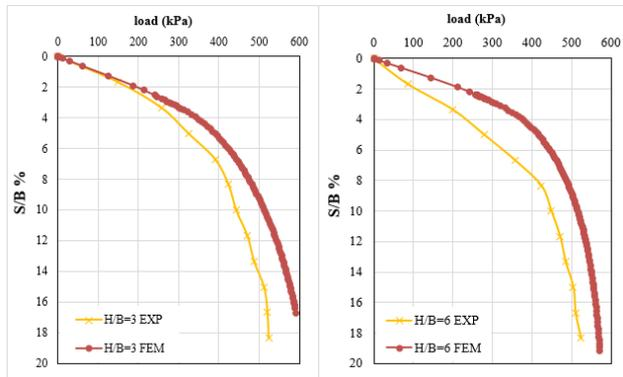
Figure 8. The experimental and numerical load-settlement curve of clay over sand layered
