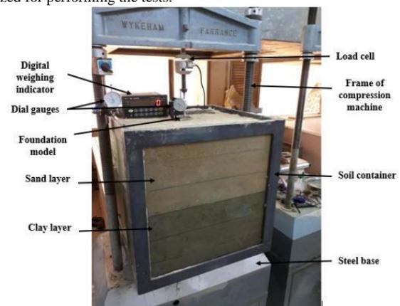
**Figure 3. The experimental setup used to perform the tests.**
