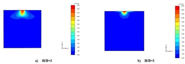
Figure 10. Failure pattern for the case of clay over-sand.
