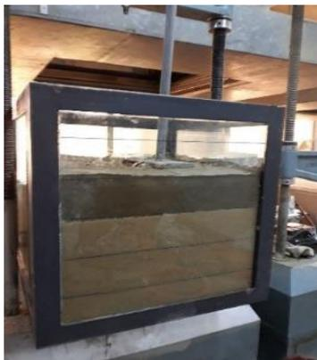
**Figure 2. Preparation of soil layered within the glass box.**
