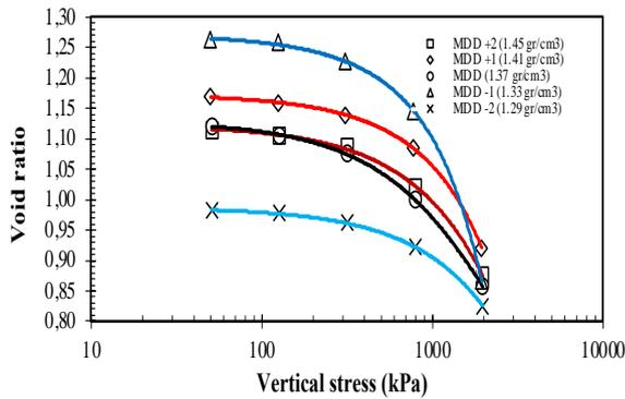
Figure 5. Consolidation Graph for LIR=1,50 on Soil Variation
