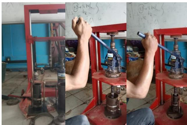
**Figure 1.** Experimental setup and the tools used to create consolidation test samples
