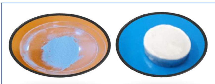
Figure 3. Silver powder before and after pressing.
