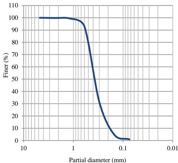
**Figure 1 - Grain size distribution curve of the sand.**
