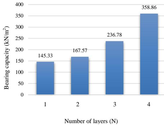
**Figure 6 - Effective of number of layers on bearing capacity**
