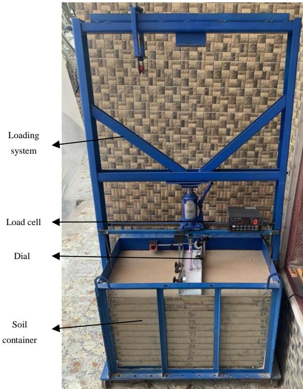
Figure 2 - Experimental set-up.
