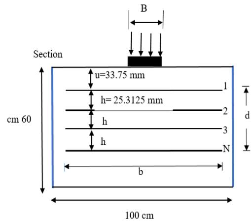
Figure 4 - Layout of geogrid spacing in cross section.
