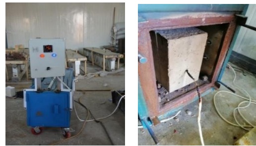
(a)Electric furnace during thermal test (b) Thermally tested RC-beam Figure 8 : Set up of the electric furnace
