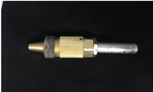
Figure 2: Zoomed image of hollow cone nozzle.
