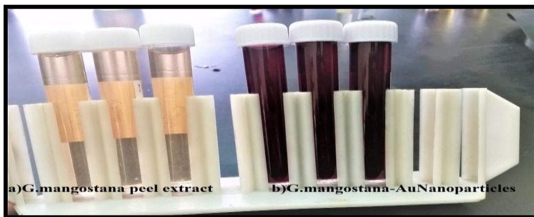
Figure (1). The color changes of G. mangostana peel extract (Left) from pale brownish into red indicating the AuNPs biosynthesis (Right).
