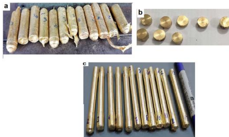
Figure 3: (a) The rod casts, (b) cutting rods to small sample and (c) Tensile test sample
