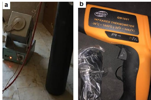
Figure 2: (a) Homogenization furnace, (b) Thermometer infrared.
