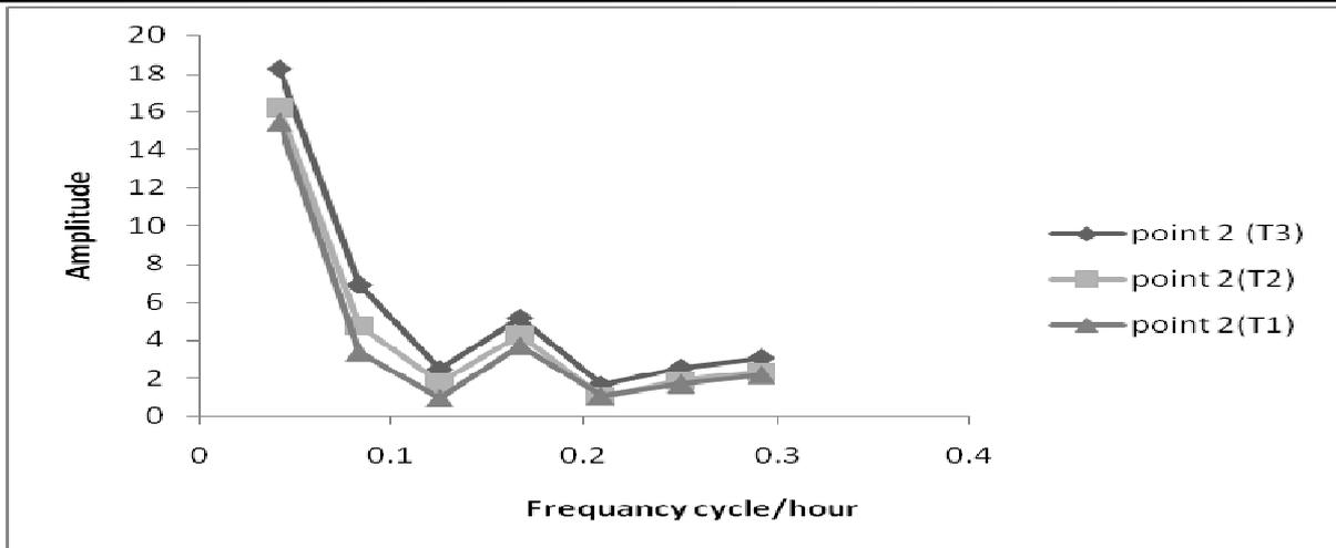
**Figure 16** change in frequency cycle per hour with amplitude ( $^{\circ}\text{C}$ ) for case with using Q-bond thermal insulation for 10 hours for sunny day
