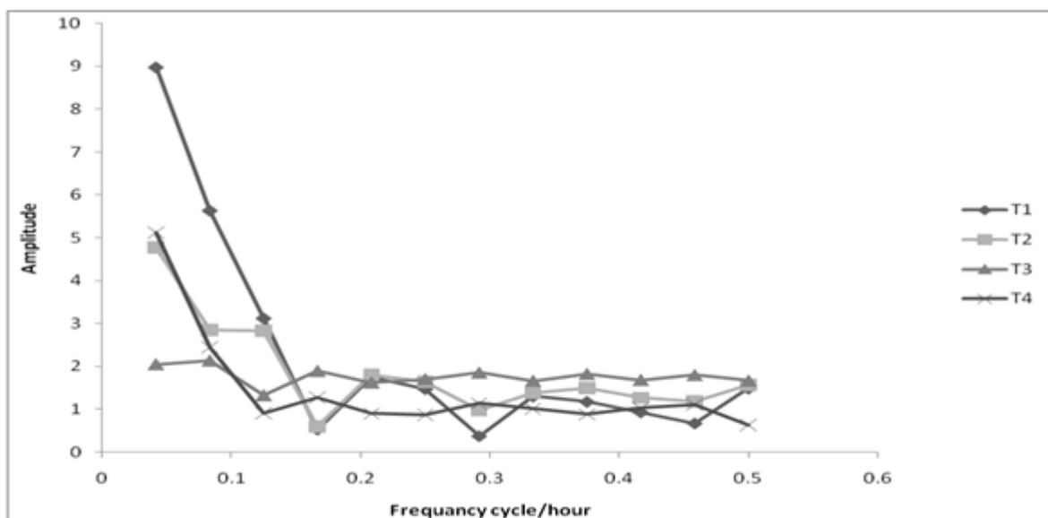
**Figure 12** change in frequency cycle per hour with amplitude ( $^{\circ}C$ ) for case with using Q-bond thermal insulation for 24 hours
