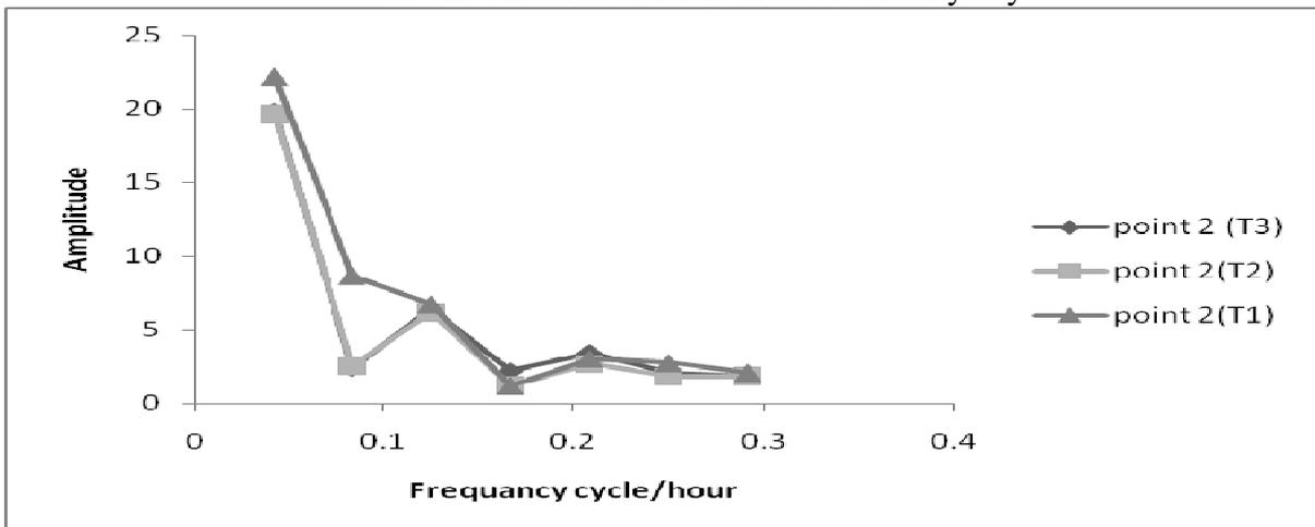
**Figure 15** change in frequency cycle per hour with amplitude ( $^{\circ}$ C) for case with using Q-bond thermal insulation for 10 hours for partly clouded day
