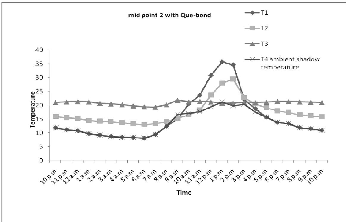
Figure 8 variation of temperature with time for sunny with Q-bond
