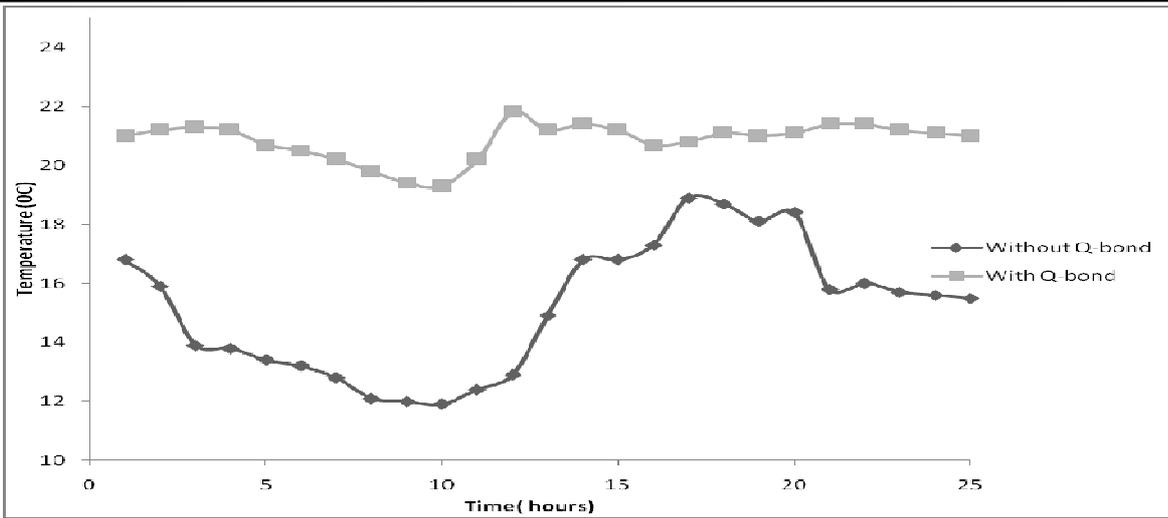
**Figure 10** Comparison between in side wall temperature ( $T_3$ ) in two cases with and without Q-bond for (24) hours.
