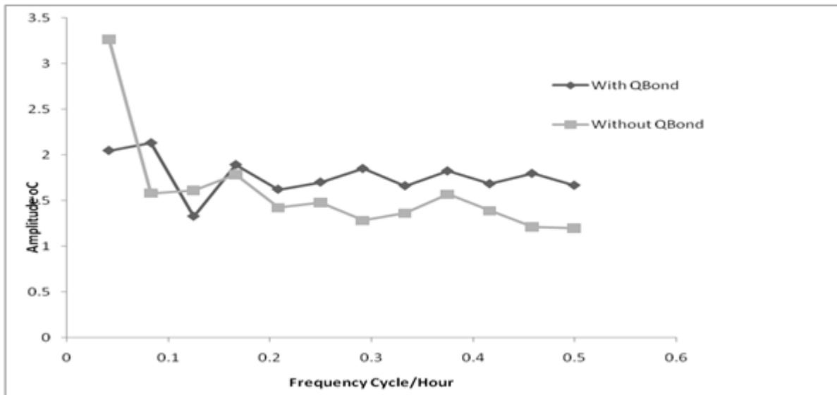
**Figure 13** A comparison between the inside wall temperatures with and without using Q-Bond thermal insulation for 24 hours
