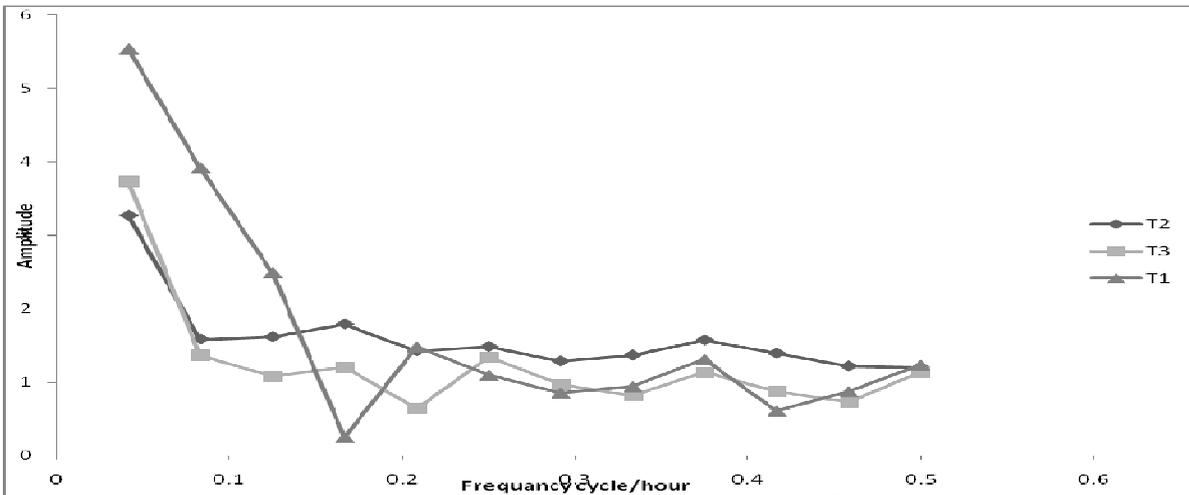
**Figure 11** change in frequency cycle per hour with amplitude ( $^{\circ}C$ ) for case without using Q-bond thermal insulation for 24 hours
