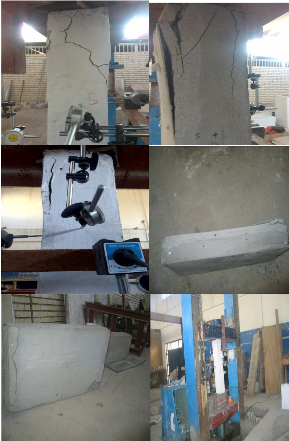
Figure 5 Buckling crack pattern for monopanel column specimens and the loading testing machine.
