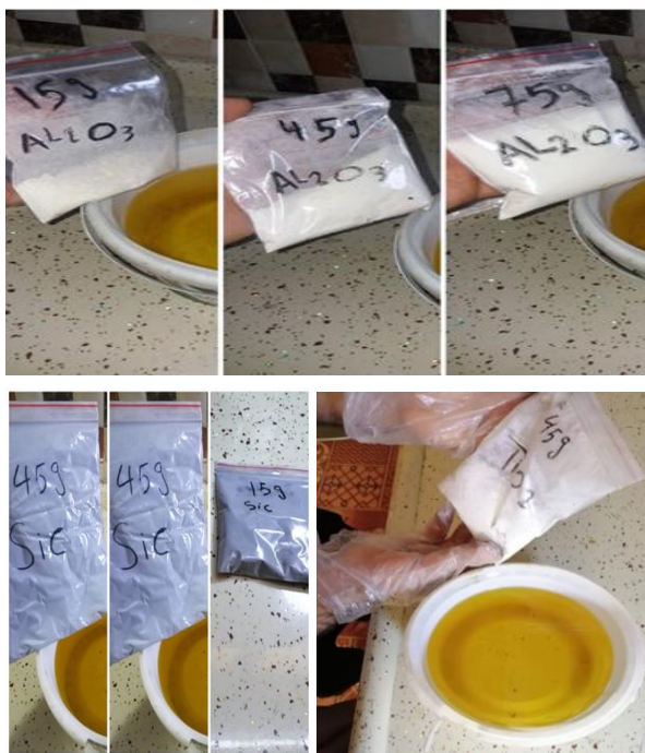
Figure 3. The stages of filling the tank with a mixture of transformer oil, paraffin wax and mineral particles
