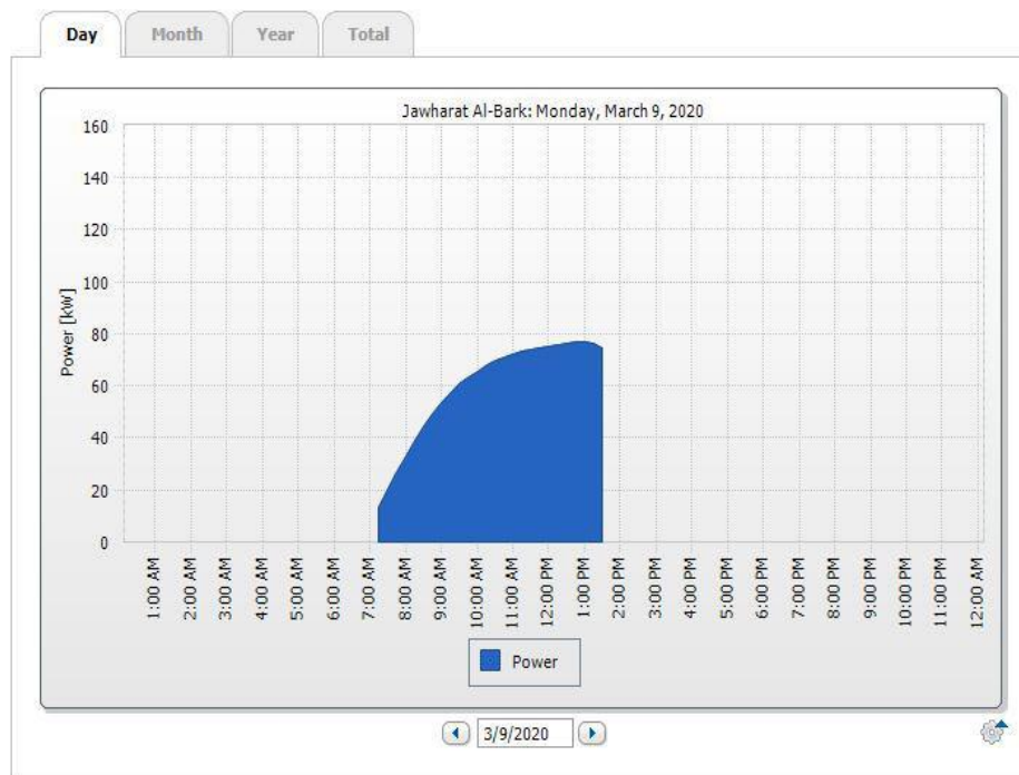
Figure 9. Actual yield of PV system in REERC building.
