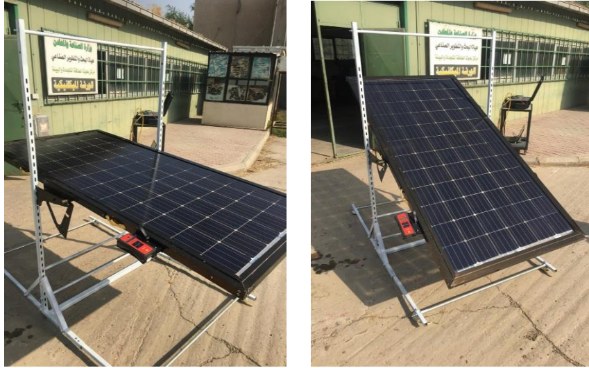
Figure (4). The bifacial solar panel oriented with two different tilt angles.
