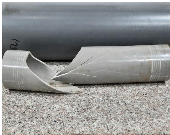
Figure (8). Cracking of PVC after rupture test.
