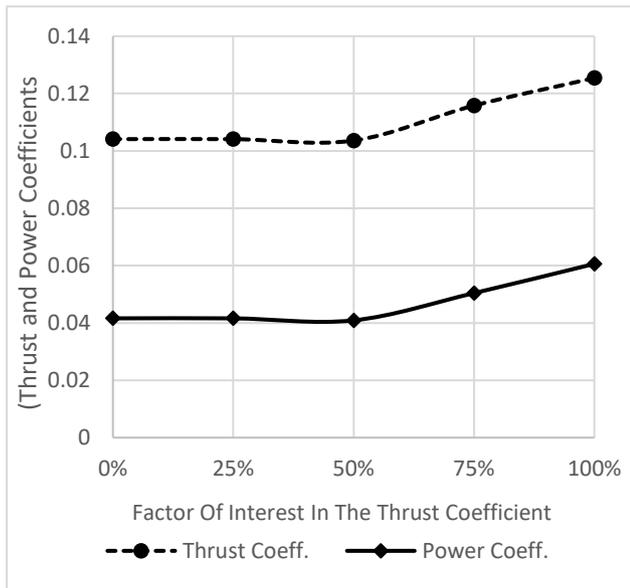
**Figure 3.** FITC vs (Thrust Coeff.) and (Power Coeff.) for Ant Colony Algorithm.
