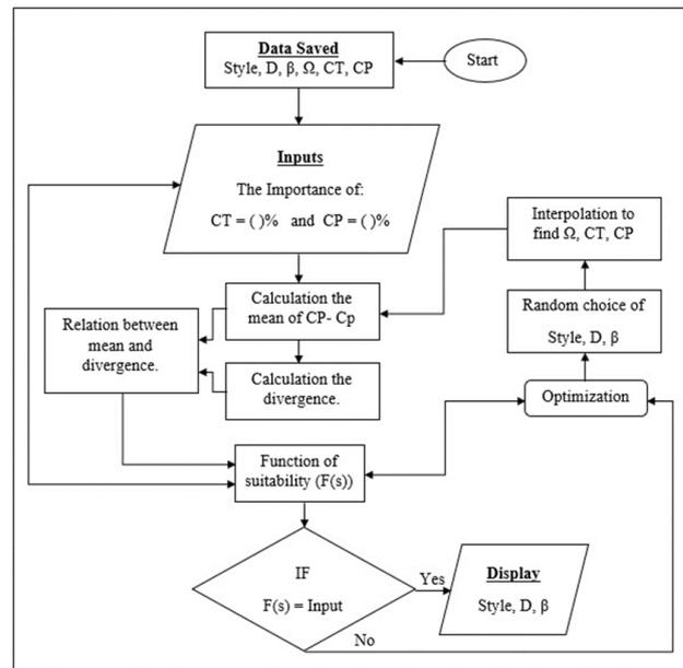
Figure 1. Flowchart for Propeller Optimization Process.
