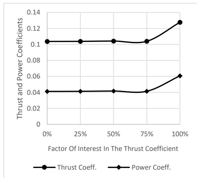
**Figure 2.** FITC vs (Thrust Coeff.) and (Power Coeff.) for Genetic algorithm.
