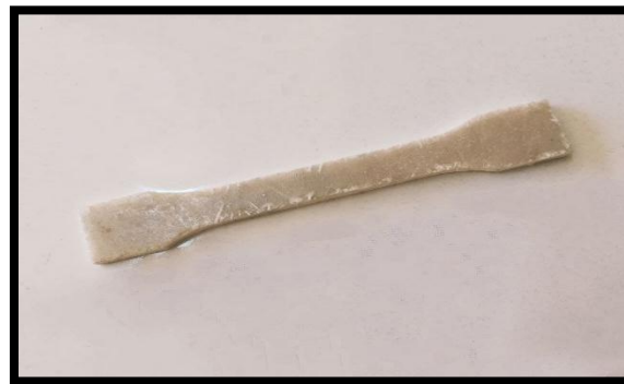
Figure (2). Tensile Test's Specimen.
