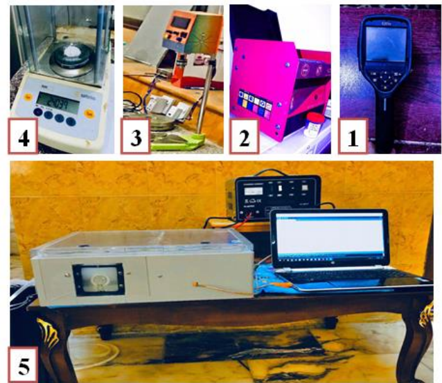
Figure 2. Experimental set-up apparatus: (1) FLIR E30bx Thermal Imaging Camera, (2) Ultrasonic waves apparatus, (3) Mechanical stirrer, (4) Sensitive balance, (5) Data logger, PC, and Test Section.
