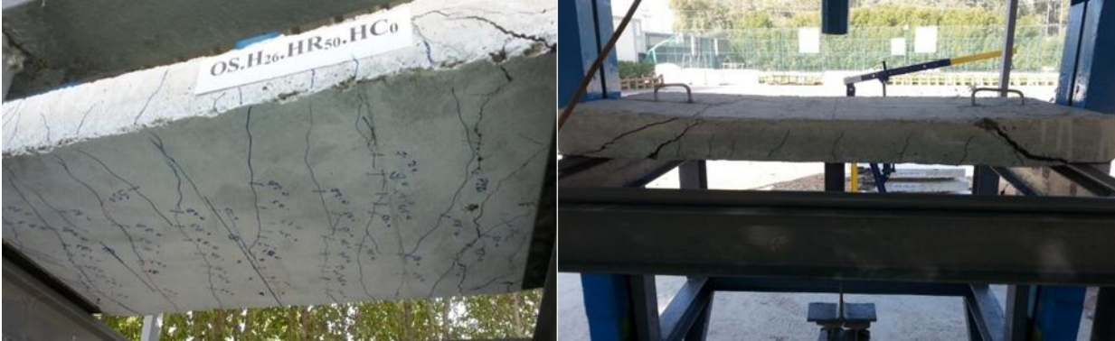
Plate 2. Mode of Failure and Cracks Pattern of Specimen OS.H26.HR50.HC0
