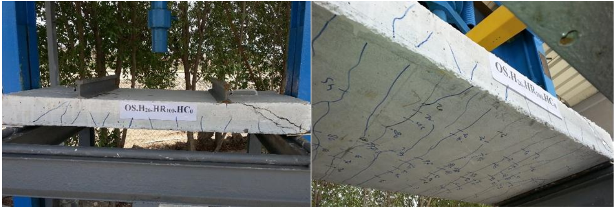
Plate 3. Mode of Failure and Cracks Pattern of Specimen OS.H26.HR100.HC0
