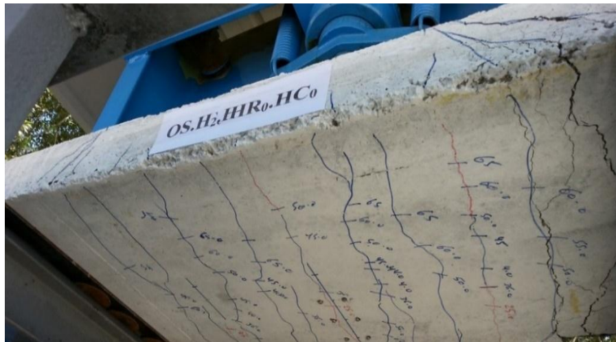
Plate 1. Mode of Failure and Cracks Pattern of Specimen OS.H26.HR0.HC0
