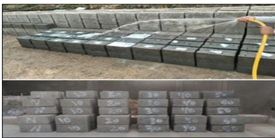
Figure 4. Water spray the rubberized concrete block samples and the final shape of the samples
