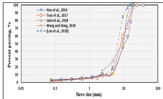
**Figure 5.** Comparison of different gradations of aggregate used for PA in some previous studies.
