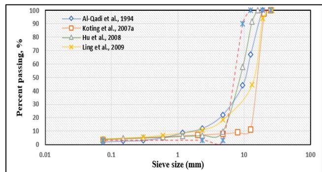
**Figure 4.** Comparison of different gradations used for PA.
