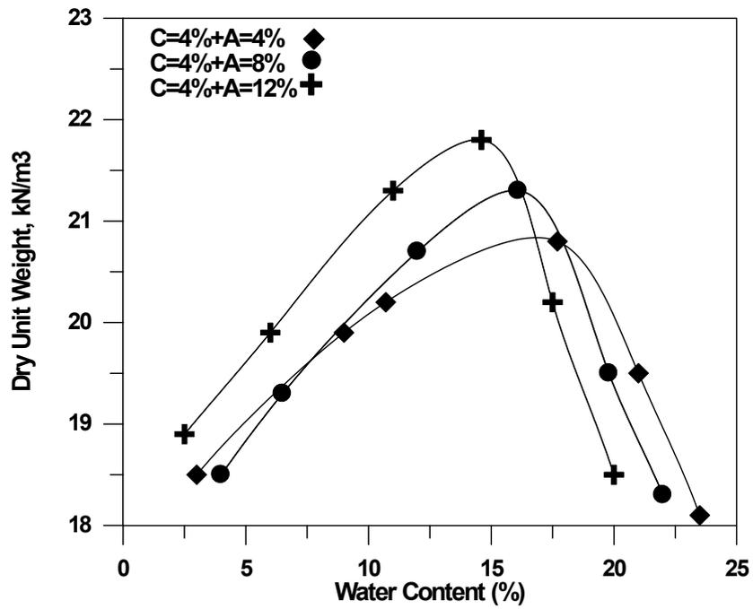
Figure (4): Standard Compaction Curves for Soil Treated with (Cement and Ceramic).
