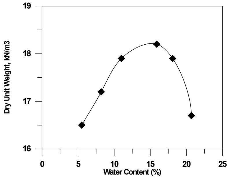
Figure (1): Standard Compaction Curve for Untreated Soil.
