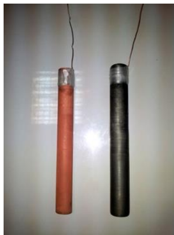
Figure 1: The cell's electrodes are the anode (copper) and the cathode (iron).
