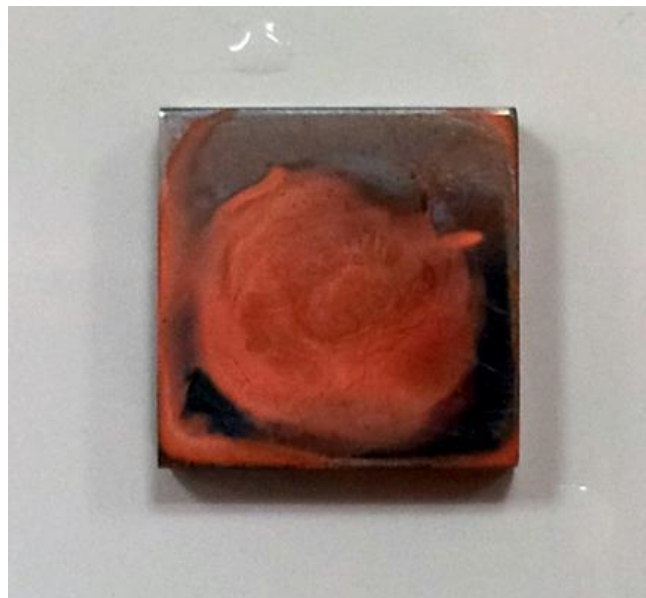
Figure 5: Iron sample after the end of the laboratory experiment using topical electroplating paste.
