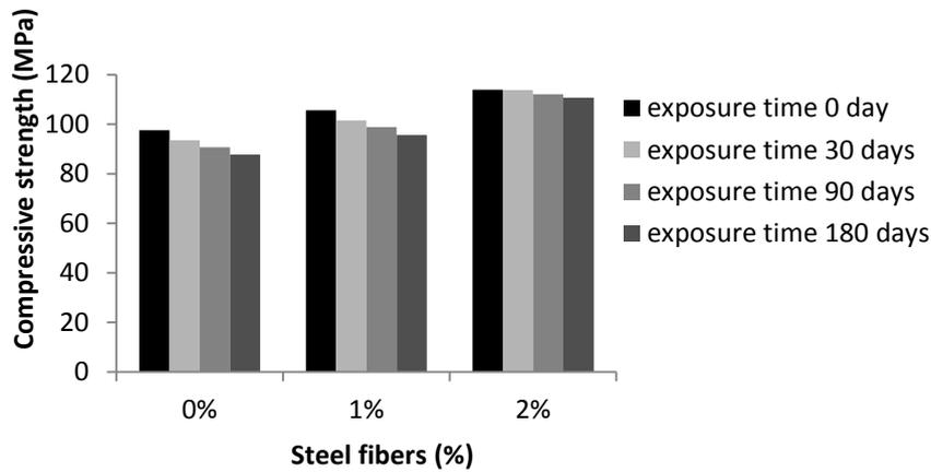
**Figure (4):** Relationship between compressive strength and steel fibers ratios of kerosene exposure
