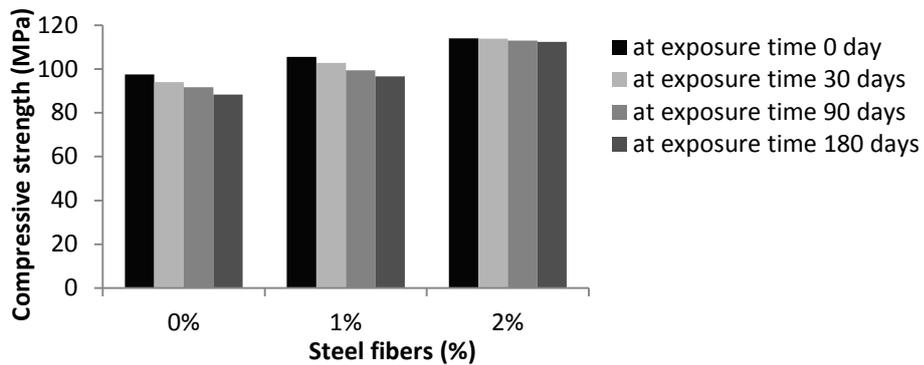
**Figure (5):** Relationship between compressive strength and steel fibers ratios of fuel oil exposure
