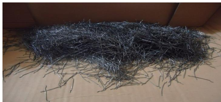
**Figure (1):** Steel Fibers used in RPC
