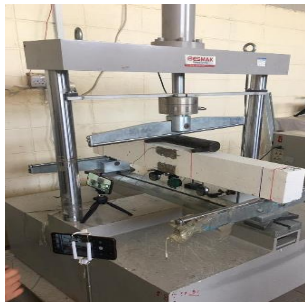
Figure .6 Experimental setup for flexural beams
