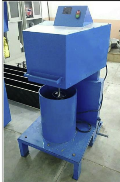
Fig. 2 The ASTM C1138/97 underwater abrasion test approach.
