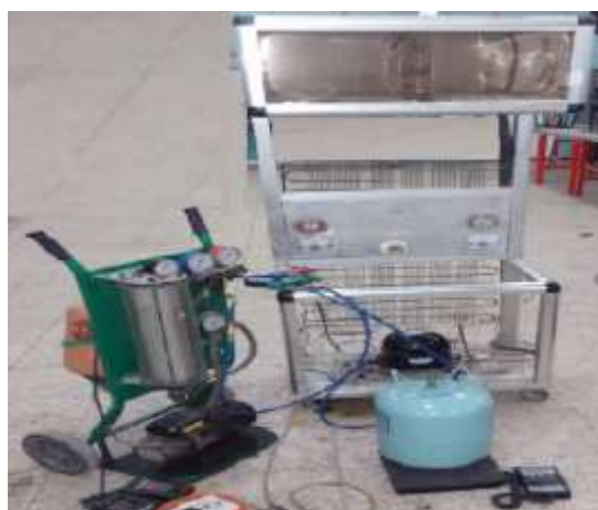
Figure (3) Refrigeration system test rig
