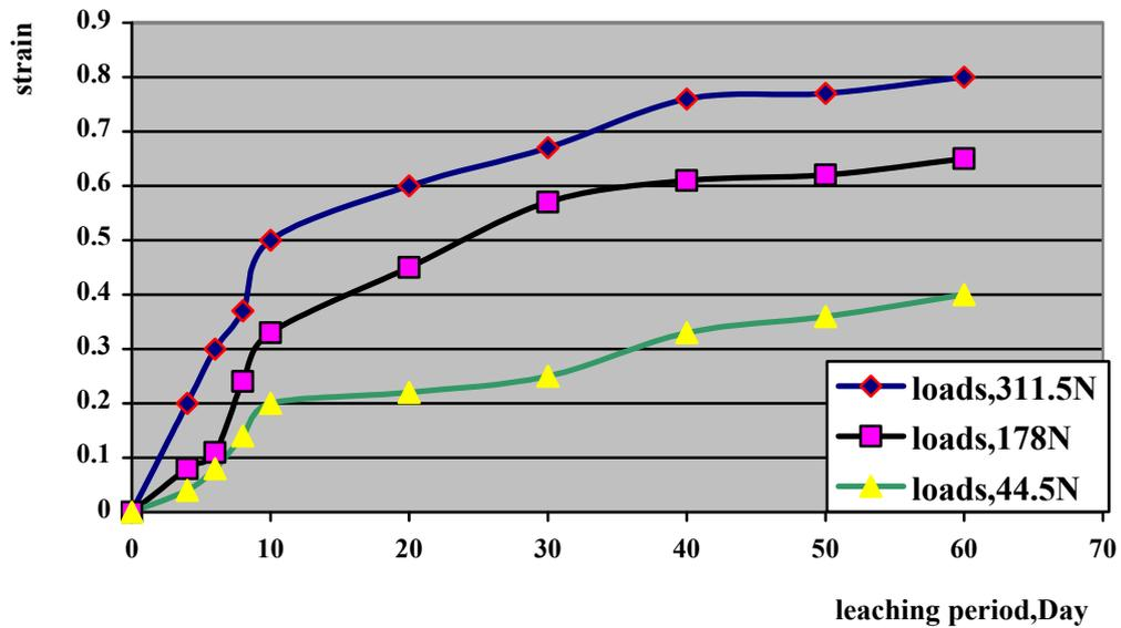
Figure (8) leaching strain versus time relation with i=10
