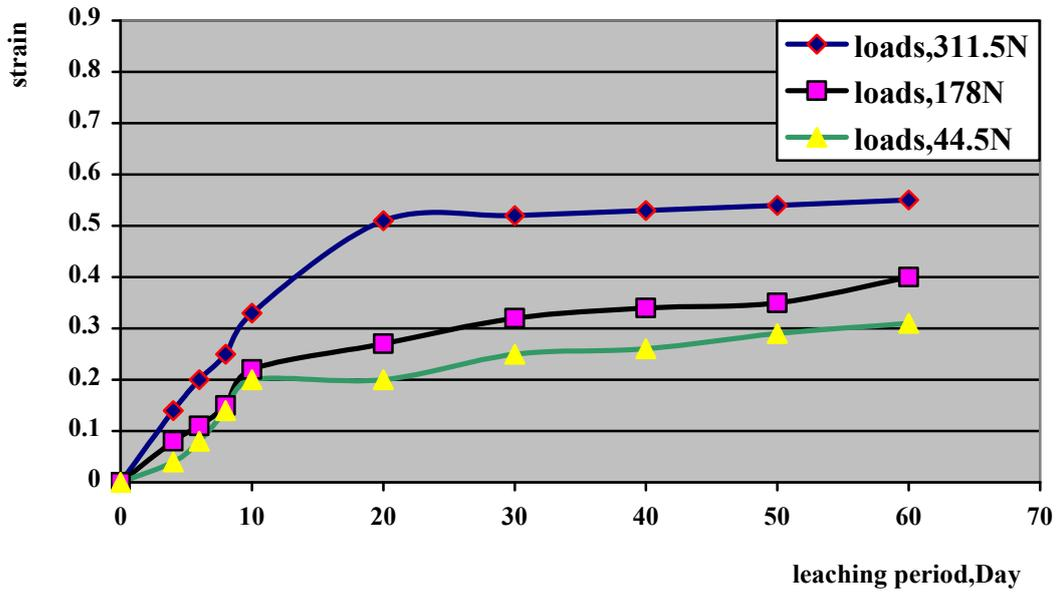
Figure (7) leaching strain versus time relation with i=6
