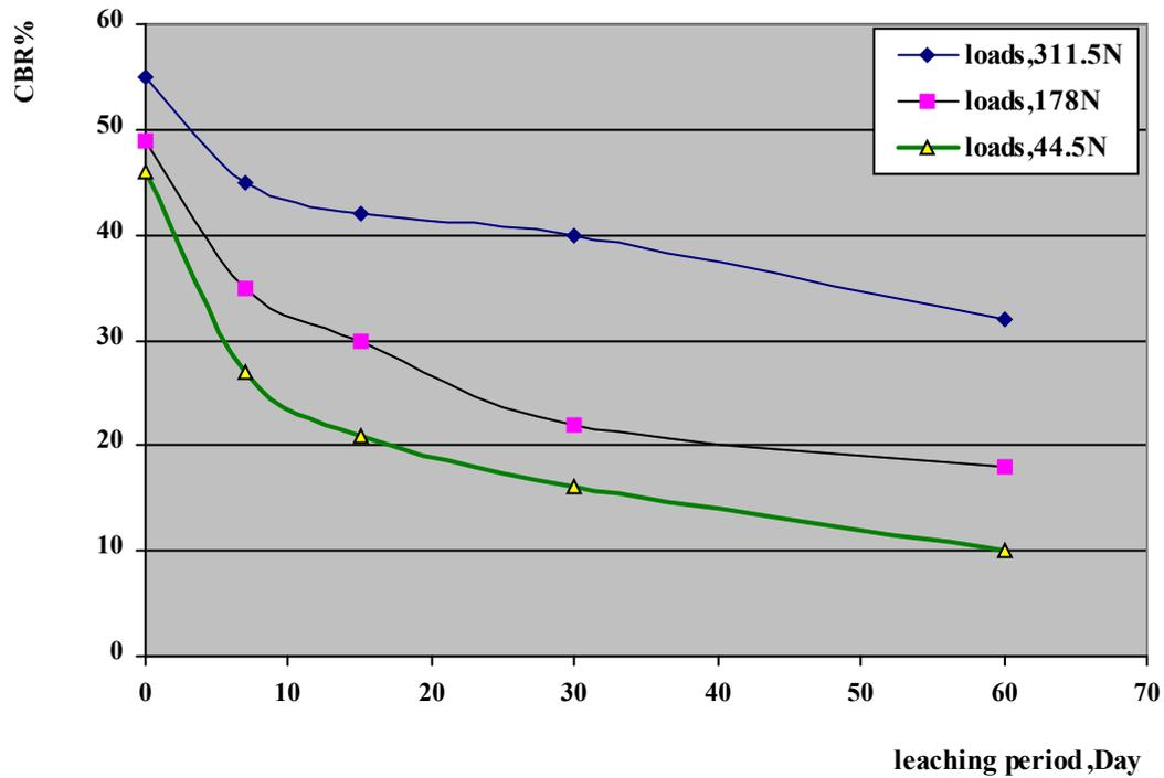
Figure(4) Effect of leaching periods on CBR under various surcharge loads with, (i=6)
