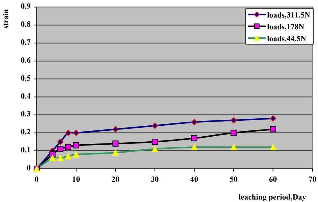
Figure (6) leaching strain versus time relation with i=2
