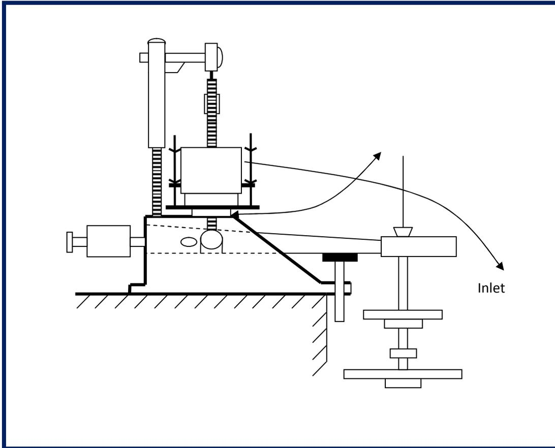
Figure (11) Arrangement of the modified oedometer
