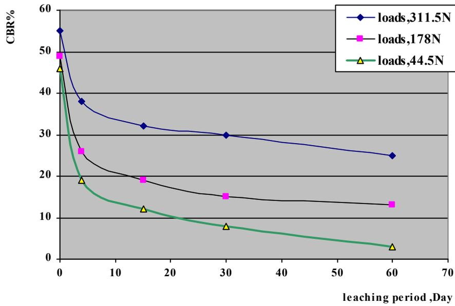
Figure(5) Effect of leaching periods on CBR under various surcharge loads with, (i=10)
