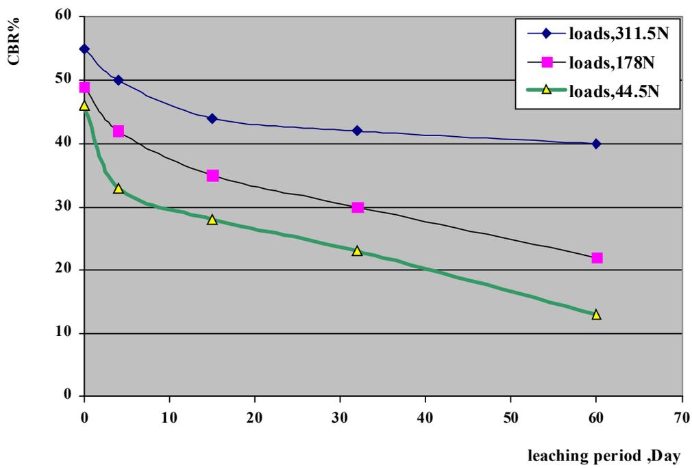
Figure(3) Effect of leaching periods on CBR under various surcharge loads with, (i=2)
