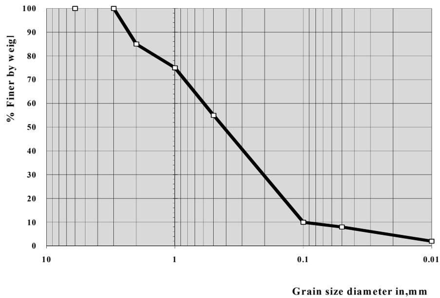
Figure 1 Grain size distribution Diagram for soils
