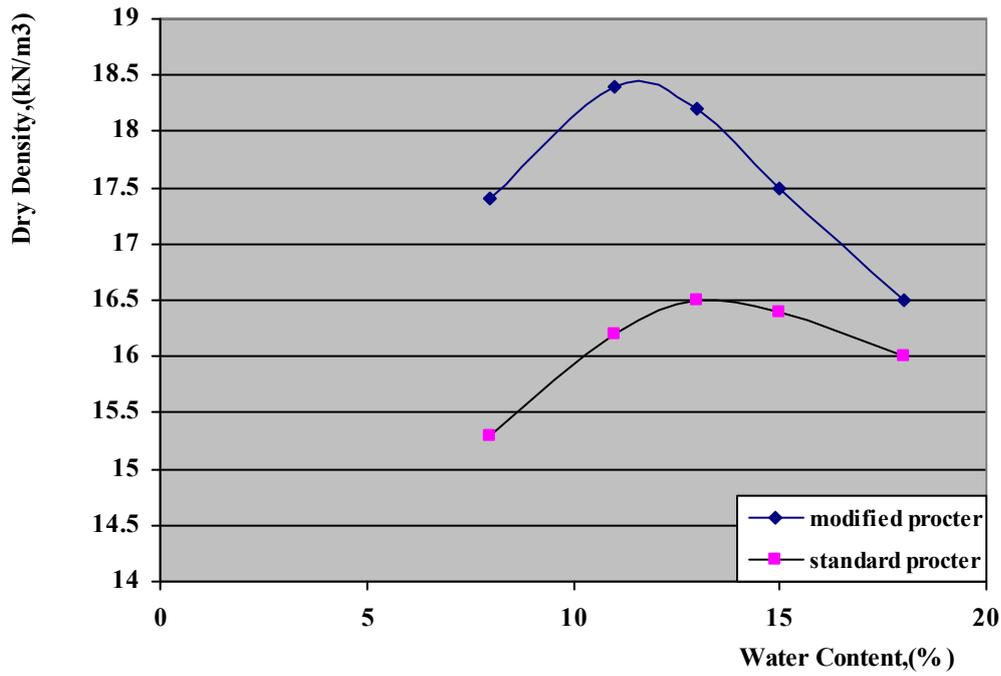
Figure (2), Procter compaction curves for samples.
