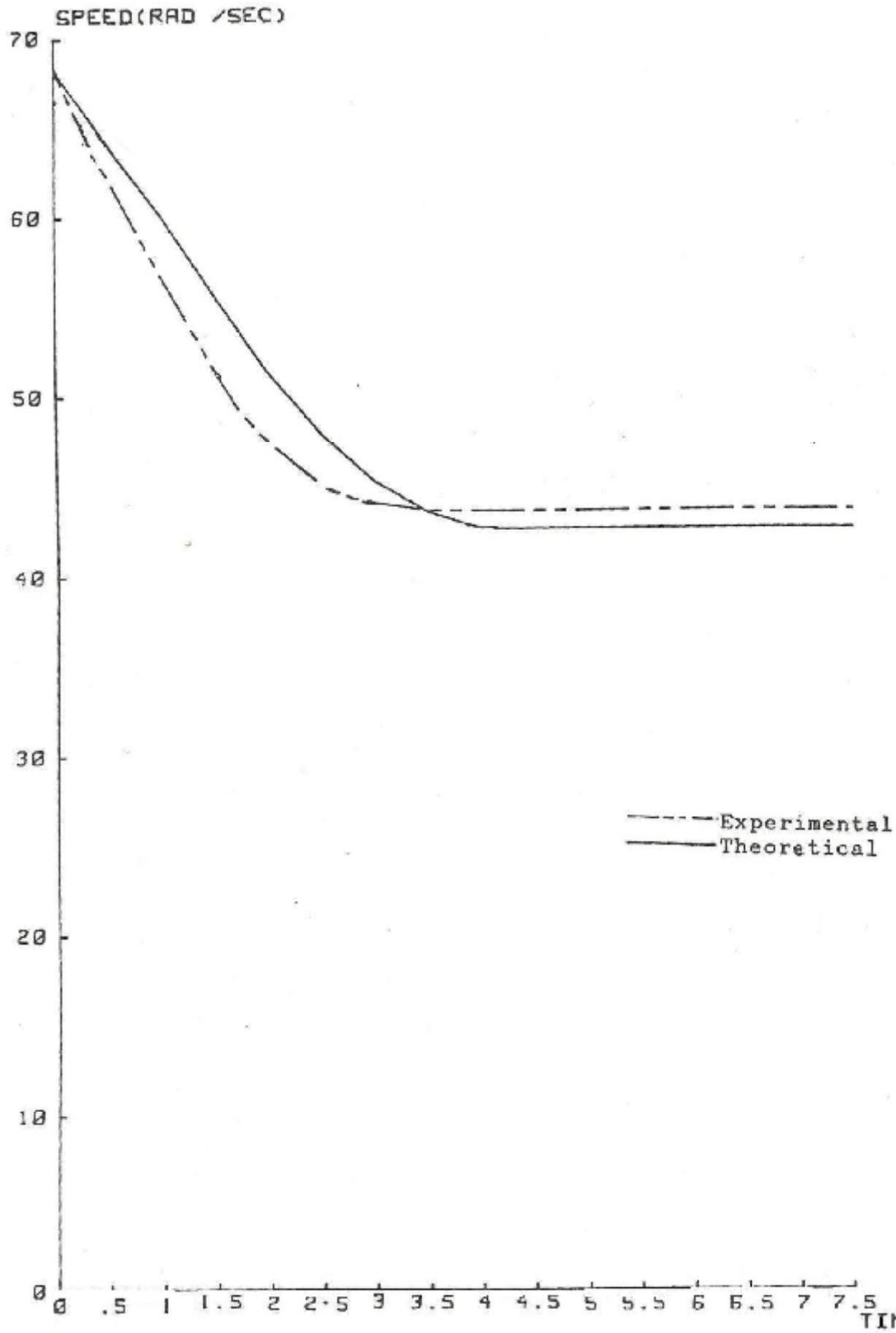
Fig.(9) Experimental and theoretical closed loop transient response of the speed for step change in reference speed  $W_r$  from 68.0 rad/sec to 44.7 rad/sec,  $W_{avo}=68.0$  rad/sec,  $i_{avo}=3.16A$ .
