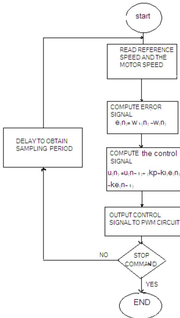
Fig.(5) The software flowchart of speed control.
