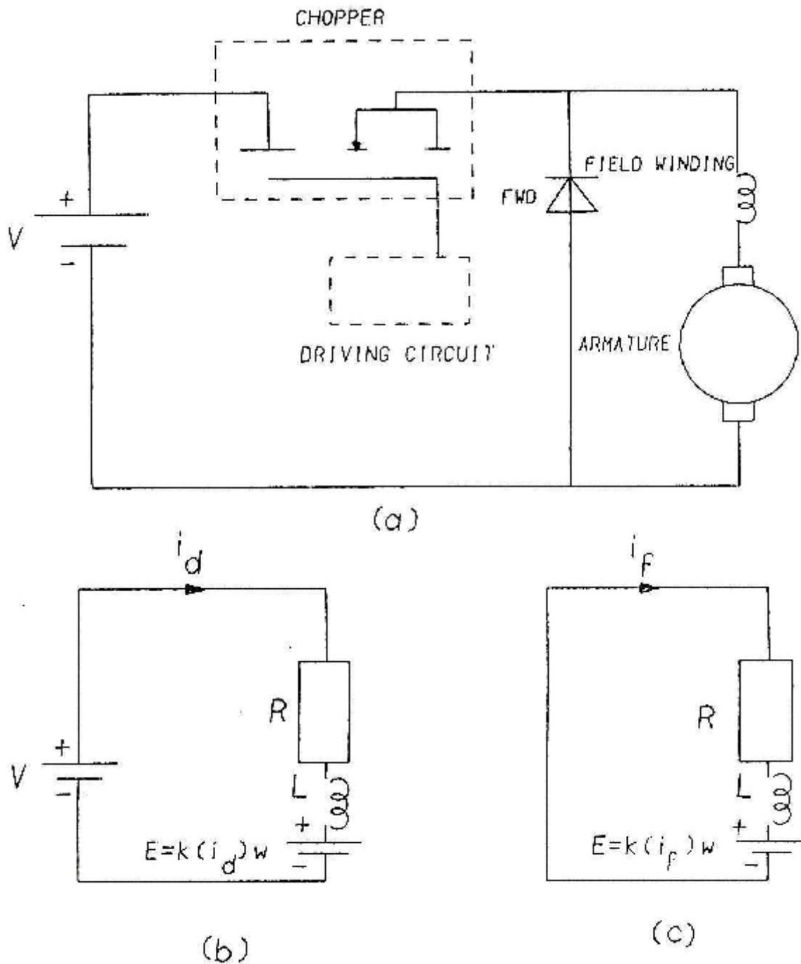
Fig.(2) Representation of a chopper – controlled dc series motor.
