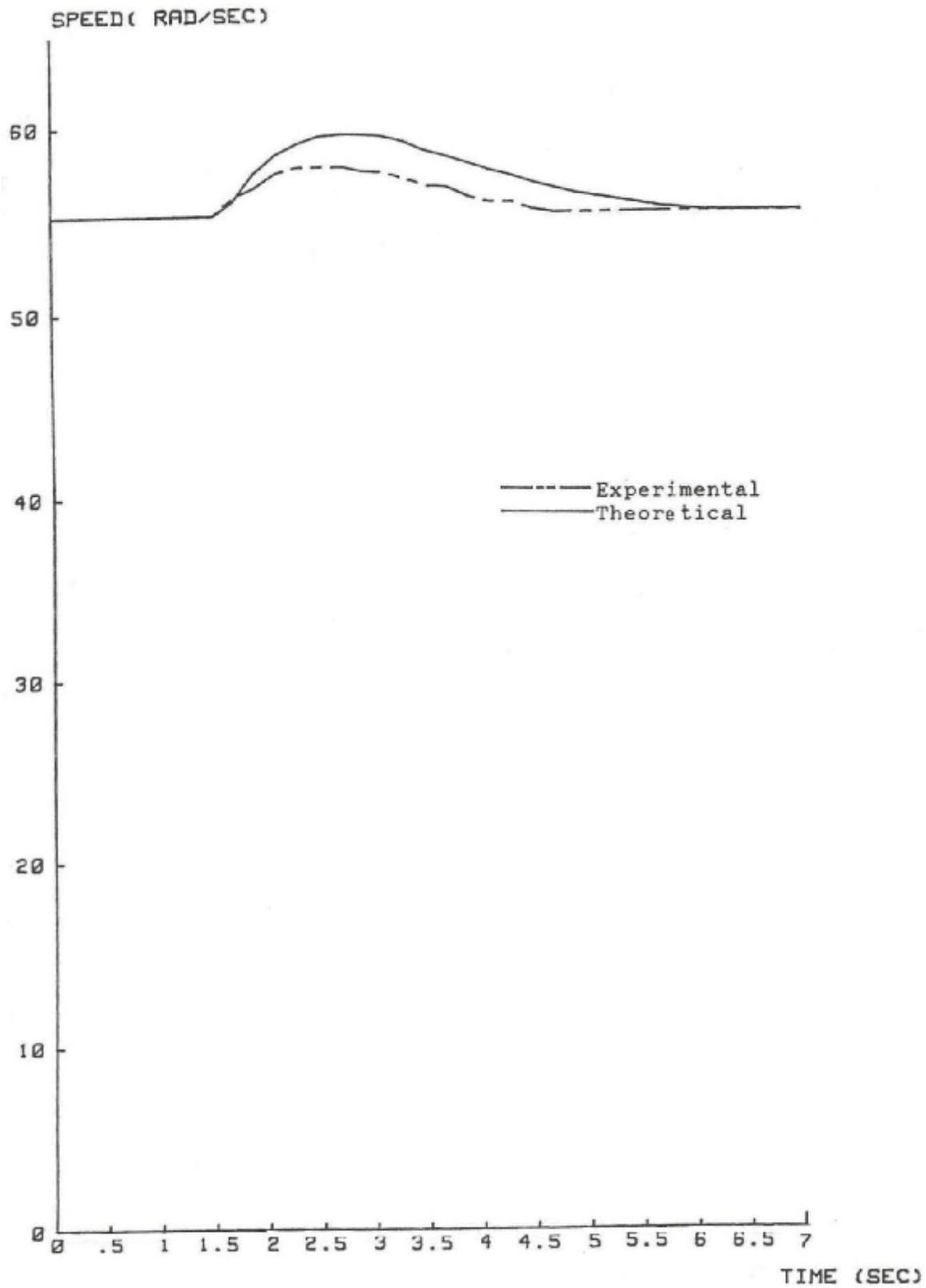
Fig.(7) Experimental and theoretical closed loop transient response of the speed for step change in load resistance  $R_L$  from  $50 \Omega$  to  $100 \Omega$  ,  $W_{avo} = 55.2 \text{ rad/sec.}$  ,  $i_{av0} = 3.38A$  .
