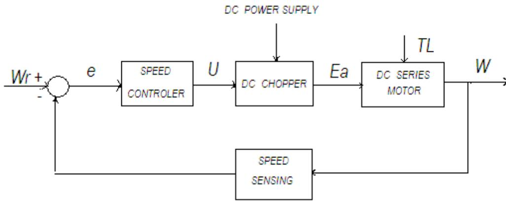
Fig.(3) Block diagram of a closed – loop fed dc series motor .
