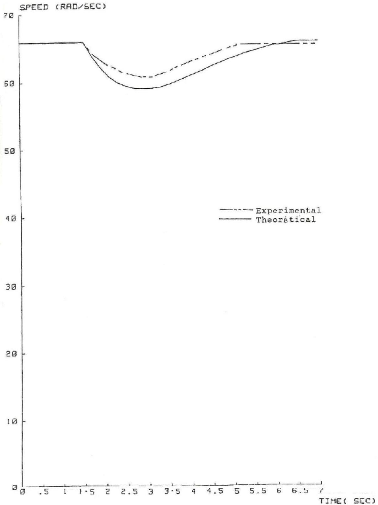
Fig.(6) Experimental and theoretical closed loop transient response of the speed for step change in load resistance  $R_L$  from  $100\Omega$  to  $50\Omega$ ,  $w_{avo} = 66.6$  rad/sec.,  $i_{avo} = 2.7A$ .
