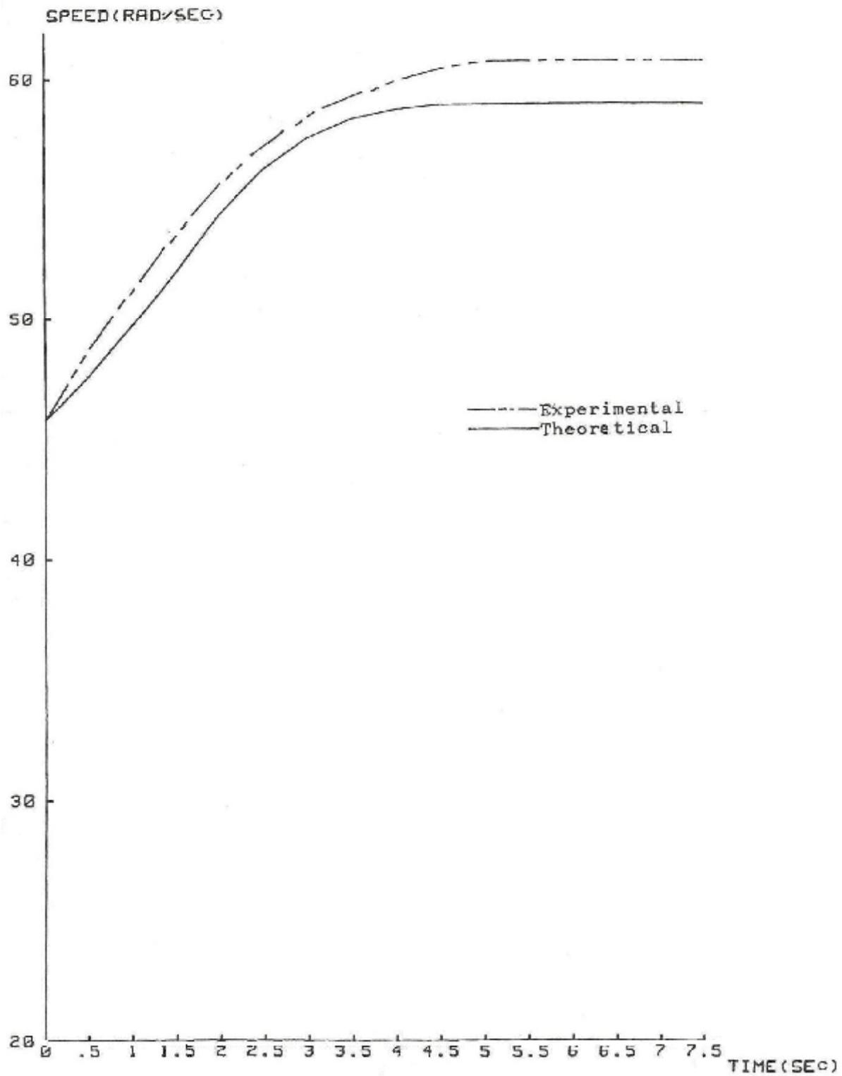
Fig.(8) Experimental and theoretical closed loop transient response of the speed for step change in reference speed  $W_r$  from 46.0 rad/sec to 59.3 rad/sec ,  $W_{avo} = 46.0$  rad/sec ,  $i_{vao} = 3.05A$  .
