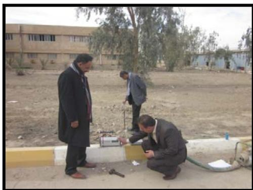
**Figure. 2 Soil and ground water radon test for well No 1.**
