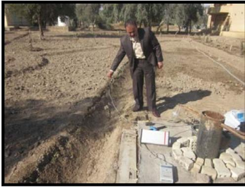
Figure. 4 Soil and ground water radon test for well No 3.
