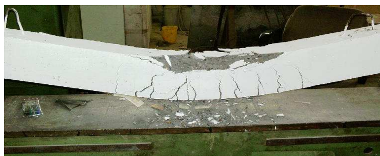
Figure 5: Deformation of beam after testing
