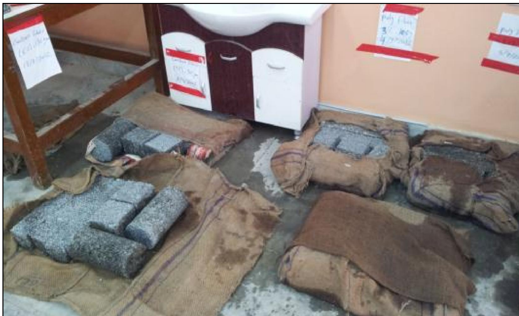
Plate 2 Curing of Concrete Samples with Wetted Gunny Sheets
