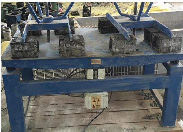
Plate 2. Vibration table (Model VV03N/2)
