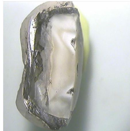
Fig.(5):-A figure representing a dye penetration for Variolink II cement in stereomicroscope at 40X magnification.
