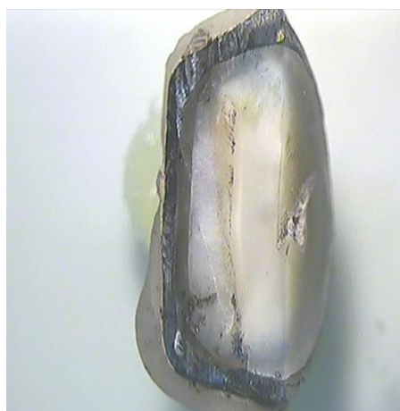
Fig.(6):- A figure representing a dye penetration for Glass ionomer cement in stereomicroscope at 40X magnification.
