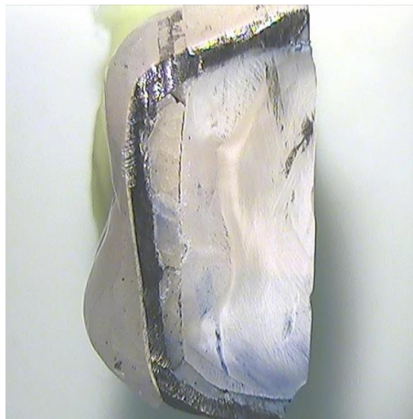
Fig.(4):-A figure representing a dye penetration for Zinc phosphate cement in stereomicroscope at 40X magnification.
