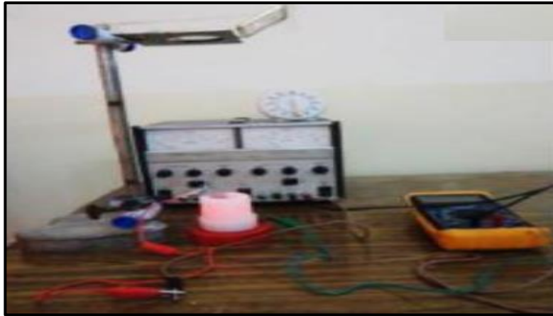
FIG. 2. PRACTICAL SETUP OF PHOTOELECTROCHEMICAL ETCHING TECHNIQUE.
