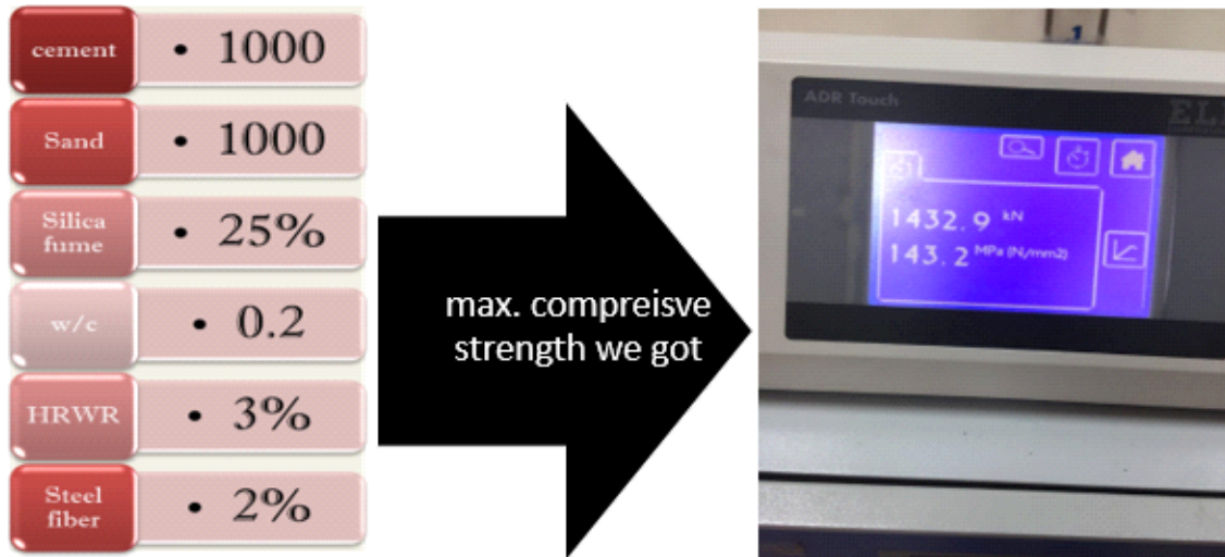
Fig.9: Mix Proportions, result compressive strength ( f_{cu} )
