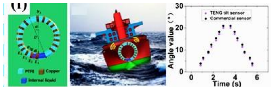
Fig. 8 A robust and self-powered tilt sensor for ship attitude sensing (Reprinted with permission from [37]. Copyright 2020 Elsevier).
