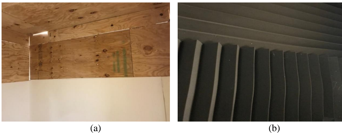
Figure 1. a) The first layer of foam (Volara Foam), b) The second layer of foam (Wedge Foam)
