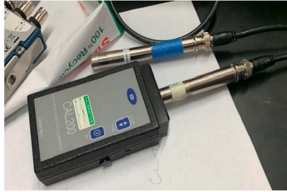
Figure 6. 1/2" Microphones as calibrated by Larson Davis CAL200
